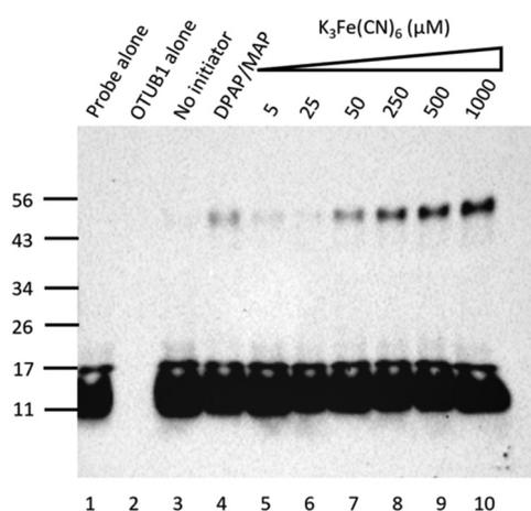
**Fig. 4** Optimisation of Fe(III) concentration for the thiol-ene labelling of OTUB1 (1  $\mu\text{g}$ ) with probe 1 (2  $\mu\text{g}$ ). Assay visualised by anti-HA Western Blotting. Samples were incubated for 90 min at 37  $^{\circ}\text{C}$ , prior to initiator addition. A mixture of DPAP and MAP was used as positive control (lane 4). Varying concentrations of potassium ferricyanide were added to lanes 5–10, which were incubated at 37  $^{\circ}\text{C}$  for 60 min.
