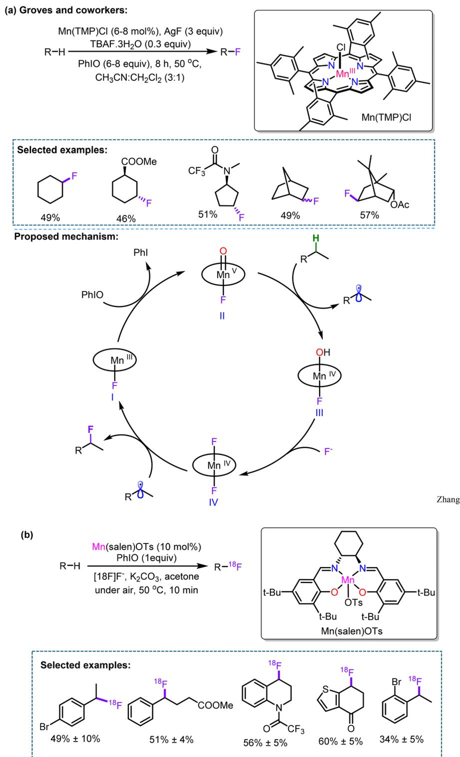
**Fig. 14** Fluorination using (a) Mn(TMP)Cl catalyst, (b) Mn(Salen)Cl catalyst, both the catalysts facilitated the transfer of fluoride to a broad range of hydrocarbons when used alongside a hypervalent iodine-based oxidant and AgF and TBAF·3H<sub>2</sub>O as fluoride sources.
