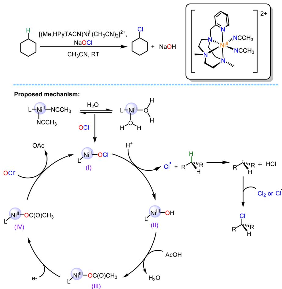
Fig. 10 Costa's catalyst for the chlorination of alkanes.
