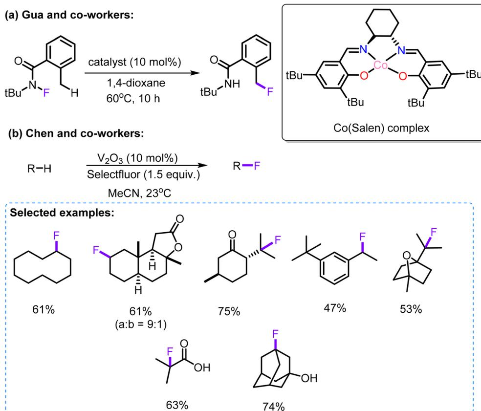
Fig. 17 C(sp<sup>3</sup>)–H fluorination using (a) Cobalt-catalyst (b) Vanadium-catalyst.
