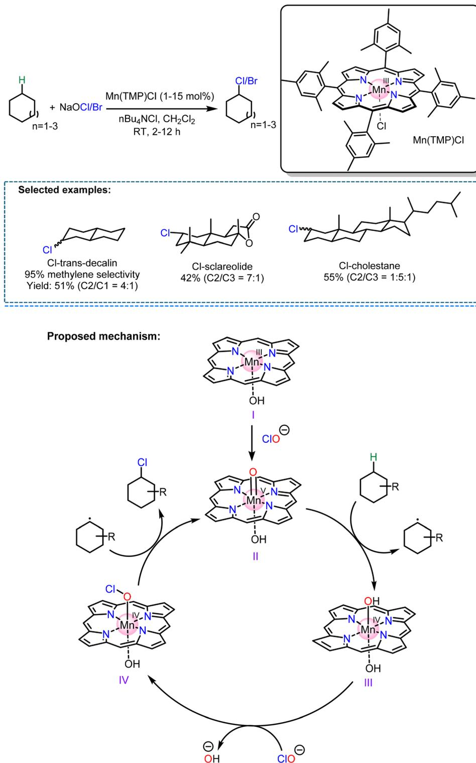
Fig. 9 Groves' catalyst for C–H chlorination and bromination.
