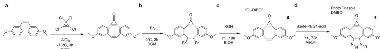
**Scheme 2** Synthesis of fluorescent triazole-DMBO, the initial step is identical to step (a) in Scheme 1. Steps a–c are adapted from Friscourt *et al.*<sup>12</sup> resulting in what they refer to as fluorescent DIBO (FL-DIBO). R = PEG1-acid.
