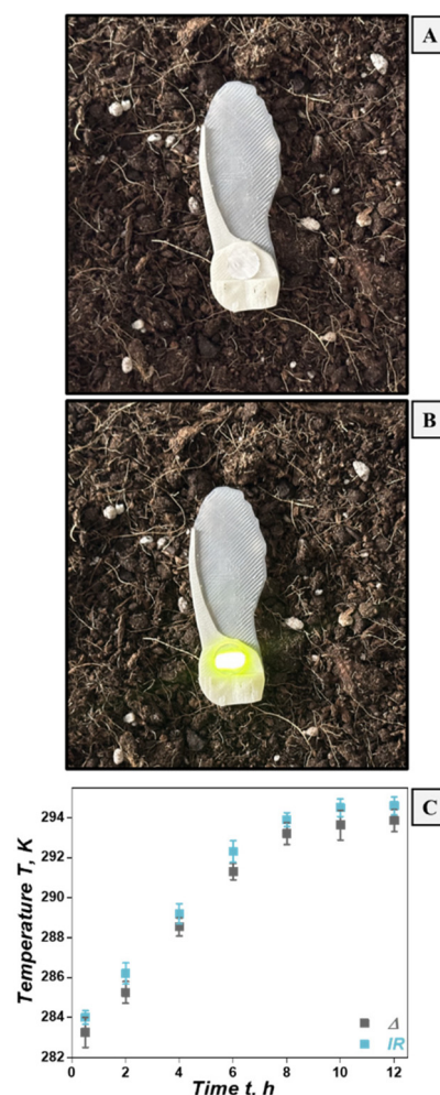
Fig. 7 Monitoring the surface temperature of topsoil with the fluorescent artificial seeds: (A) on topsoil, (B) irradiated with a 980 nm laser, and (C) temperature of the topsoil determined from the fluorescent seeds ("Δ" in gray) and from a reference external infrared thermometer ("IR" in blue).
