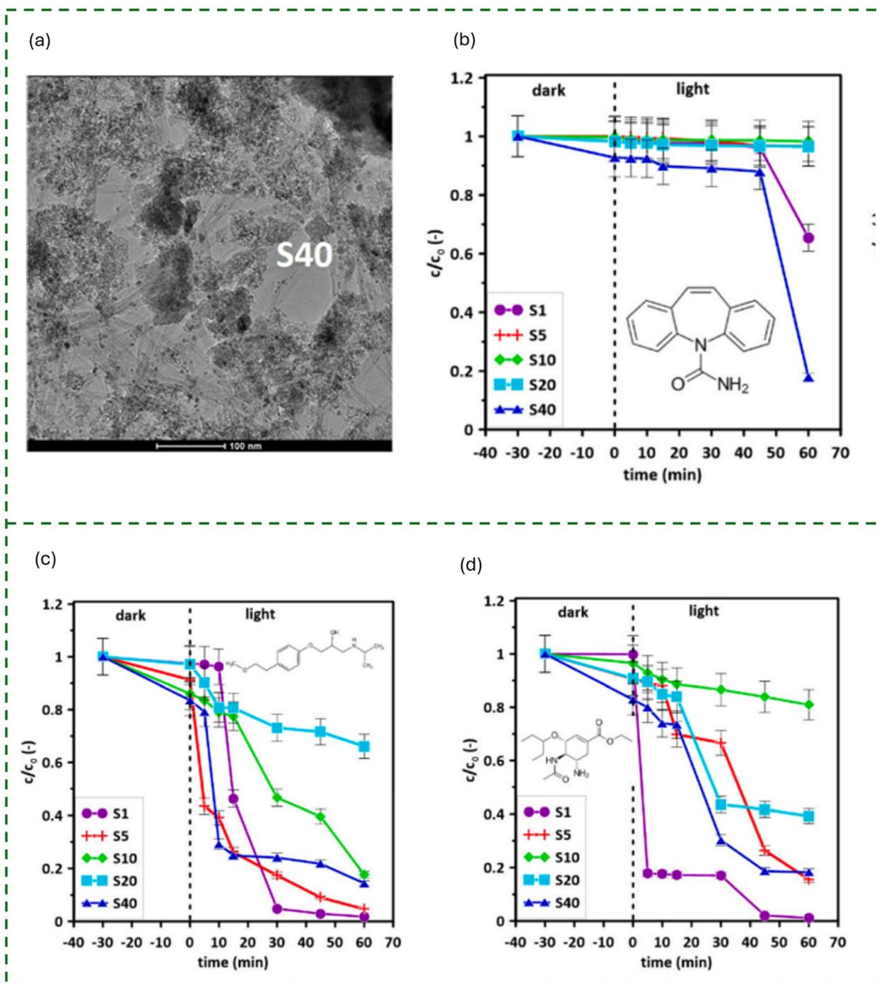
Fig. 14 (a) Surface characteristics of SWCNT-TiO<sub>2</sub>/SiO<sub>2</sub> nanocomposites. Kinetics of PPCPs (pharmaceutical and personal care products) photocatalytic removal: (b) IBU (ibuprofen), (c) MET (metoprolol), and (d) OSA (oseltamivir).<sup>171</sup> Figures a–d reprinted from ref. 171 *J. Photochem. Photobiol., A*, 2025, 467, 116437, with permission from Elsevier, copyright 2026.
