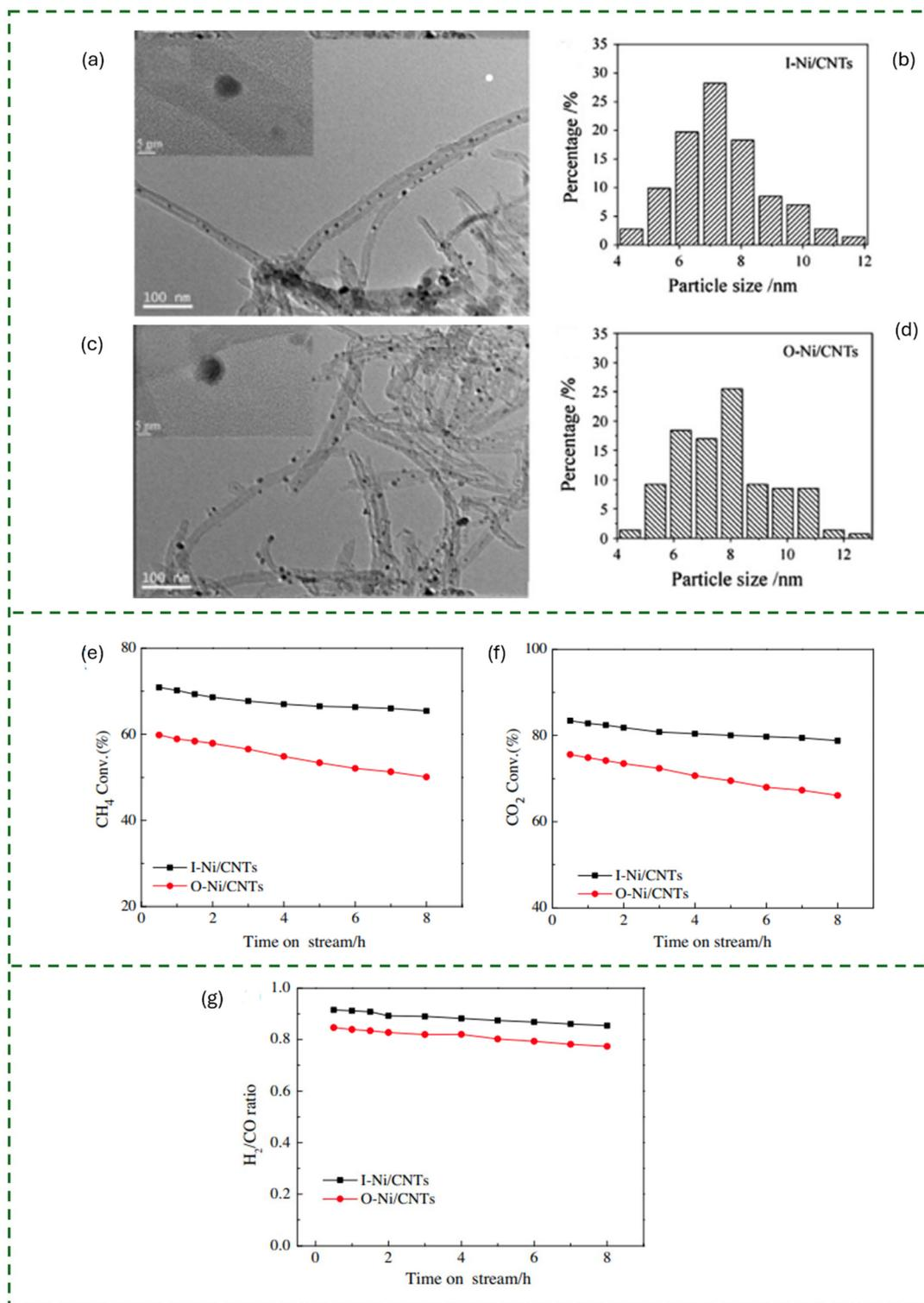
**Fig. 10** TEM images and particle size distribution of (a, b) I-Ni/CNTs and (c, d) O-Ni/CNTs. Catalytic stability of I-Ni/CNTs and O-Ni/CNTs: (e) CH<sub>4</sub> conversion; (f) CO<sub>2</sub> conversion; (g) H<sub>2</sub>/CO ratio. (Reaction conditions: 750 °C, W/F = 1 g h mol<sup>-1</sup>.)<sup>9</sup> Figures a–g reprinted from ref. 9 *Fuel*, 2013, **108**, 430–438, with permission from Elsevier, copyright 2026.
