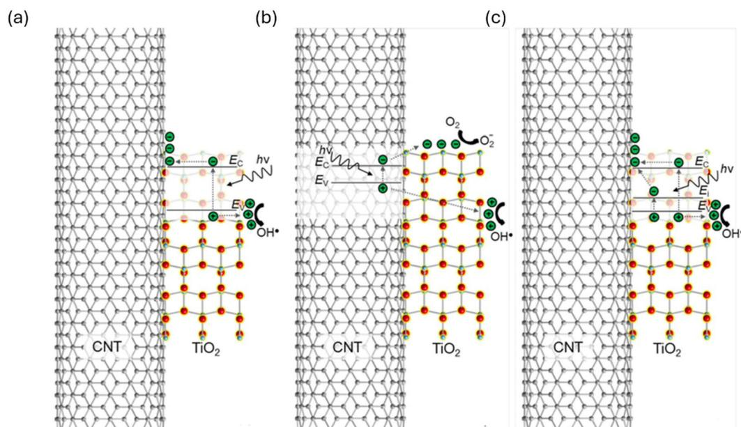
**Fig. 11** Mechanism of TiO<sub>2</sub>-CNT composite. (a) electron scavenging, (b) photosensitization, and (c) band-gap modification.<sup>166</sup> Figures a–c reprinted from ref. 166 *Beilstein J. Nanotechnol.*, 2014, 5, 946–955.
