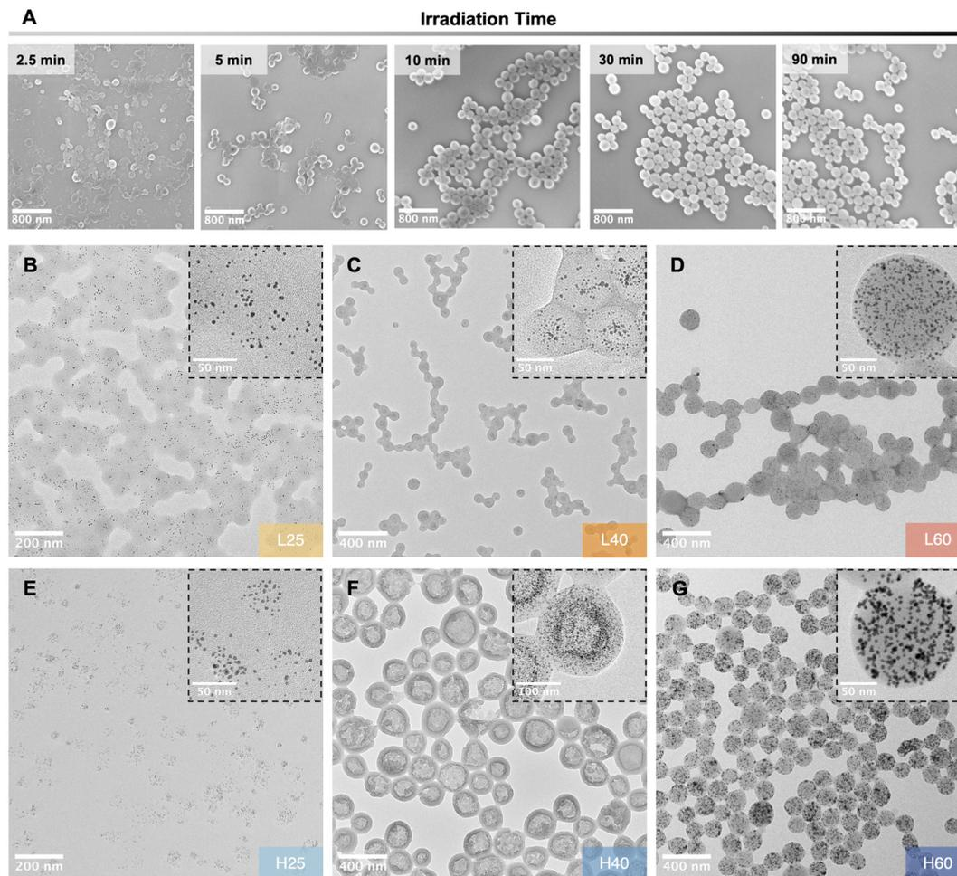
**Fig. 1** (A) SEM images of H40 samples synthesized with different irradiation times. TEM images of the hybrid nanogels synthesized at different reagent concentrations and temperatures. Panels show (B) L25, (C) L40, (D) L60, (E) H25, (F) H40, and (G) H60.
