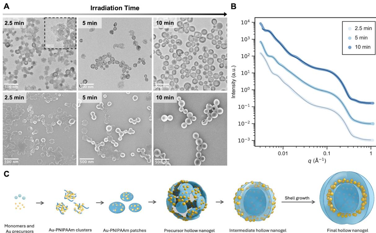
**Fig. 2** Investigation of hollow nanogel formation in H40. (A) TEM (upper row) and SEM (lower row) images of H40 irradiated for 2.5, 5, and 10 minutes. (B) SAXS data of H40 at 2.5, 5, and 10 minutes fitted with a combined core-shell, sphere, and Guinier model. (C) Proposed mechanism of hollow nanogel formation.
