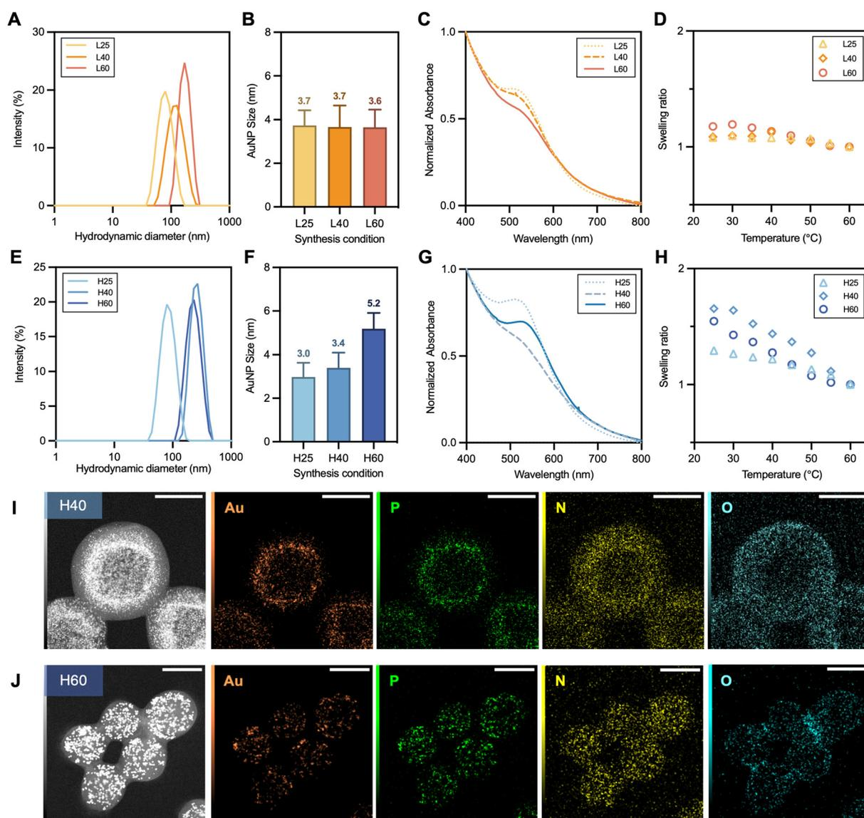
**Fig. 3** Characterization of the synthesized hybrid nanogels. (A and E) Hydrodynamic diameters of L-series and H-series measured by DLS. (B and F) AuNP sizes of L-series and H-series determined from TEM images ( $n = 300$ ). (C and G) UV-Vis spectra of L-series and H-series. (D and H) Temperature-dependent swelling ratios of L-series and H-series measured by DLS from 25 °C to 60 °C at 5 °C intervals. (I and J) EDS elemental maps (Au, P, N, and O) for H40 (I) and H60 (J) (scale bar = 100 nm).
