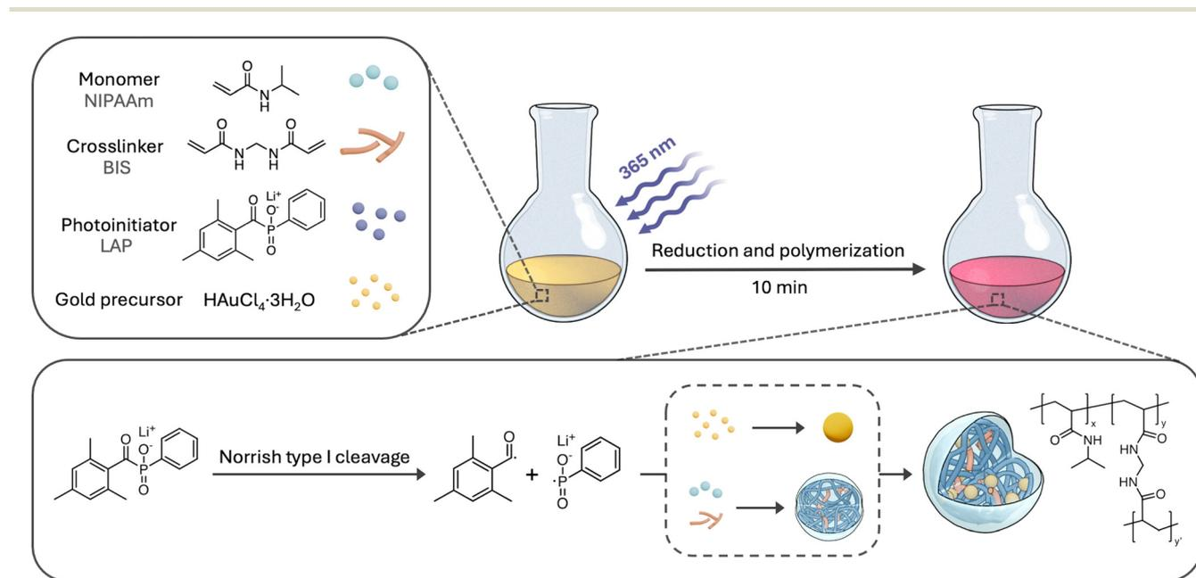
**Scheme 1** Schematic of Au–PNIPAAm hybrid nanogel synthesis *via* a single-step photochemical approach. The photoinitiator LAP undergoes Norrish type I cleavage to generate radicals that drive simultaneous reduction, polymerization, and crosslinking within 10 minutes, yielding polymer nanogels with AuNPs embedded in the networks.
