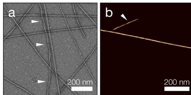
**Fig. 1** Micrographs showing amyloid fibrils formed by VQIVYK following prolonged incubation. (a) TEM shows a major population of smooth fibrils and fewer with a pronounced twist. (b) AFM shows very long smooth fibrils and a smaller population of twisted fibrils made up of protofilaments. White arrows highlight twisted fibrils in (a) and (b).
