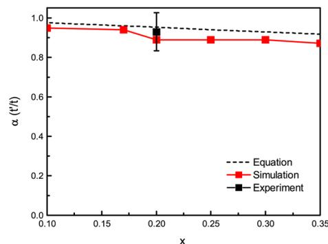
Fig. 7 Comparison of the oxide length ratios ( $\alpha$ ) obtained from simulations and experiments compared with the calculations from eqn (2)–(4).  $x$  represents the Ge content relative to Si in the SiGeO alloy. For the experimental results, the error bar denotes the standard deviation ( $\pm 0.1$ ).
