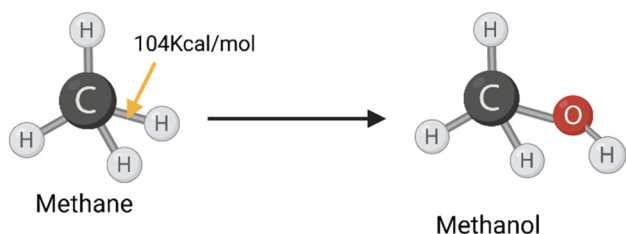
Fig. 17 Schematic representation of methane to methanol oxidation.
