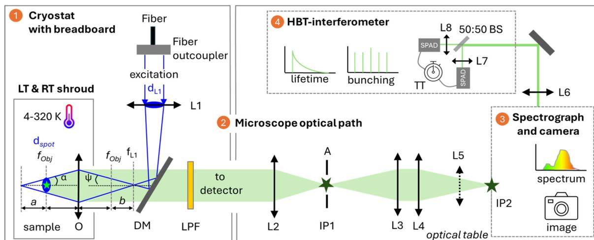
**Fig. 1** Schematic of the cryo-optical setup with components indicated: (1) cryostat with a breadboard and a shroud hosting a sample and a low-temperature objective (O), (2) microscope optical path (IP – image plane), (3) spectrograph and camera for spectroscopy, imaging, and spectral selection, and (4) HBT-interferometer. For abbreviations of optical components and variables, see Table 1 and eqn (1)–(3), respectively.
