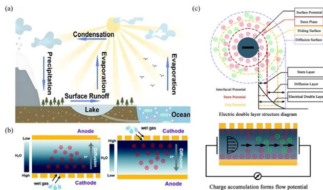
**Fig. 2** (a) Illustration of abundant and sustainable moisture in the environment.<sup>5</sup> Reproduced from ref. 5 with permission from Elsevier, copyright 2022. (b) Schematic diagram of ion gradient diffusion mechanism.<sup>25</sup> Reproduced from ref. 25 with permission from Royal Society of Chemistry, copyright 2018. (c) Streaming potential mechanism diagram.
