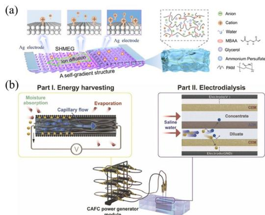
**Fig. 7** (a) Schematic illustration of the preparation and structure of SHMEG.<sup>89</sup> Reproduced from ref. 89 with permission from John Wiley and Sons, copyright 2025. (b) Schematic of a hybrid ED system coupled with stacked cellulose acetate fiber columns (CAFC) power generators.<sup>90</sup> Reproduced from ref. 90 with permission from Elsevier, copyright 2024.
