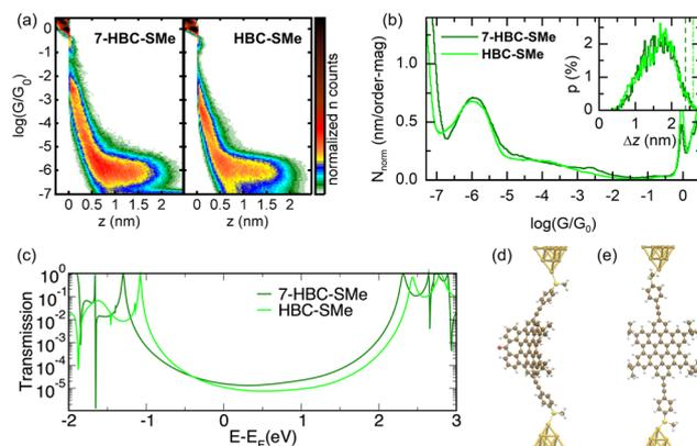
**Fig. 2** 2D (a) and 1D (b) histograms for 7-HBC-SMe and HBC-SMe. They were built with all the traces displaying plateaus from the different measurement rounds performed for these molecules. Inset in (b) corresponds to the plateau-length distributions. Transmission versus Energy ( $E$ ) curves calculated for 7-HBC-SMe and HBC-SMe (c), in the electrode-molecule-electrode configuration depicted in (d) and (e), respectively.
