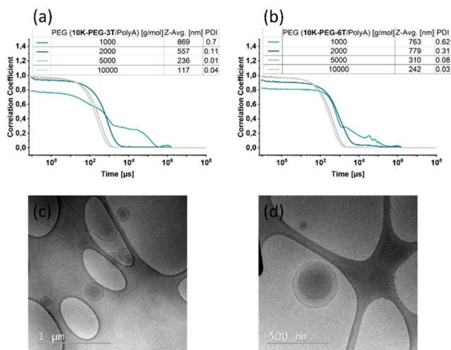
**Fig. 3** DLS measurements to investigate the influence of PEG chain length on the nanoparticle formation of PEG-3T/polyA (a), and PEG-6T/polyA (b). The concentrations of PEG-3T and PEG-6T were 80  $\mu$ M and the polyA concentration was 720  $\mu$ M. The solvent used was 1× PBS. The table shows the mean value of the Z-average and the PDI of three individual measurements. Cryo-TEM images of 5K-PEG-3T/polyA. The sizes of the scale bars are 1  $\mu$ m (c) and 500 nm (d).
