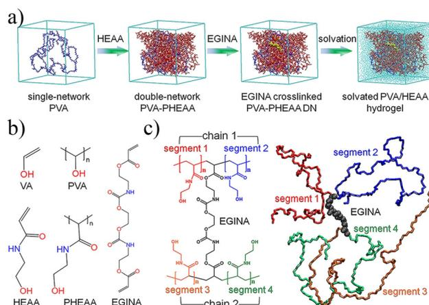
**Fig. 6** Multiscale construction of crosslinked hydrogel networks for molecular simulations. (a) Stepwise modelling pipeline to build solvated double-network hydrogels from monomer structures and crosslinkers. (b and c) Molecular structures and 3D representations of the polymer chains and EGINA crosslinking topology. Adapted from Liu *et al.*<sup>193</sup>
