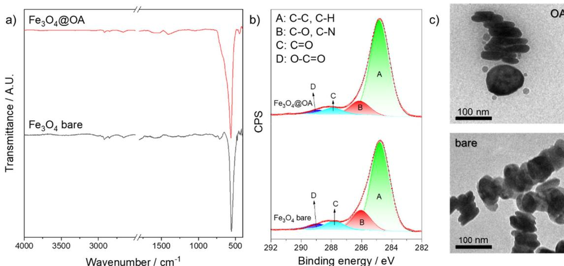
Fig. 2 Characterization of Fe<sub>3</sub>O<sub>4</sub>@OA and bare Fe<sub>3</sub>O<sub>4</sub> by (a) FTIR, (b) XPS corresponding to the C 1s region, and (c) TEM (top: Fe<sub>3</sub>O<sub>4</sub>@OA; bottom: bare Fe<sub>3</sub>O<sub>4</sub>).
