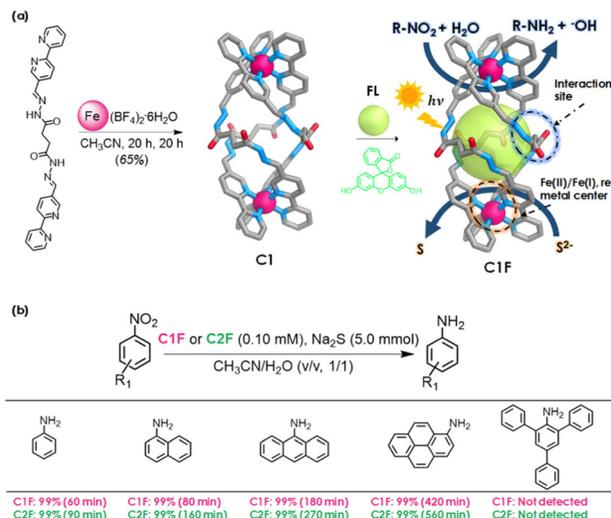
**Fig. 7** (a) Schematic representation of self-assembly of **C1** and the photocatalytic system of **C1F** for the combination of H<sub>2</sub>S splitting and hydrogenation of nitroaromatics. (b) Photocatalytic reduction of different nitroaromatics into aminoarenes under standard conditions: substrate (0.50 mmol).
