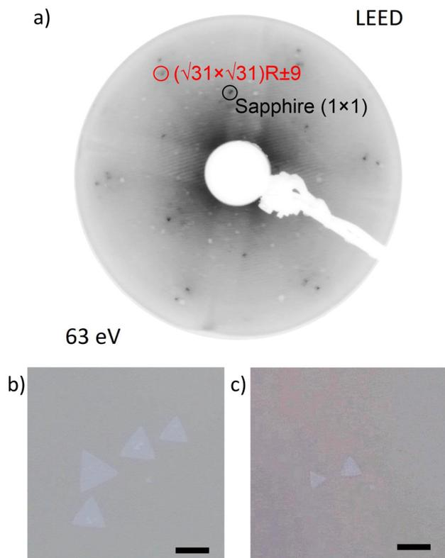
**Fig. 1** H<sub>2</sub>-annealing of sapphire. (a) Diffraction pattern of H<sub>2</sub>-annealed sapphire measured by LEED at 63 eV, showing the  $(\sqrt{31} \times \sqrt{31})R \pm 9^\circ$  surface reconstruction. (b) WS<sub>2</sub> crystals grown on H<sub>2</sub>-annealed sapphire. (c) WS<sub>2</sub> grown on *standard* sapphire. The scale bars are 20  $\mu\text{m}$ .
