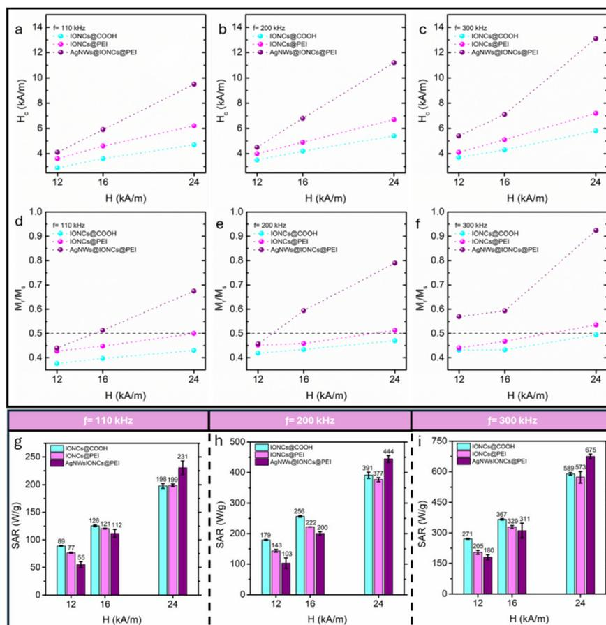
**Fig. 5** Evaluation of  $H_c$  (a–c) and  $M_s/M_r$  (d–f) values as a function of applied magnetic field strength at various frequencies. The SAR values of IONCs@COOH, IONCs@PEI, and AgNWs@IONCs@PEI at various magnetic field strengths and frequencies of 110 (g), 200 (h), and 300 kHz (i).
