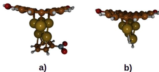
Fig. 5 (a) NB ( $E_{\text{ads}} = -1.53$  eV) and (b) H<sub>2</sub> ( $E_{\text{ads}} = -0.76$  eV) adsorption on Ni atoms in RGO@Ni.
