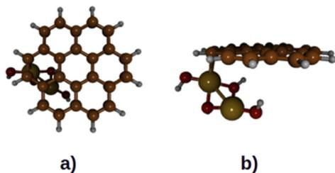
Fig. 2 (a) Top and (b) side view of the optimized structure of RGO@Ni(OH)<sub>2</sub>.
