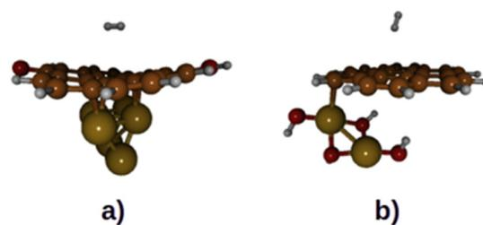
Fig. 3 H<sub>2</sub> adsorption on top of RGO in the presence of (a) RGO@Ni ( $E_{\text{ads}} = -0.07$  eV) and (b) RGO@Ni(OH)<sub>2</sub> ( $E_{\text{ads}} = -0.07$  eV).
