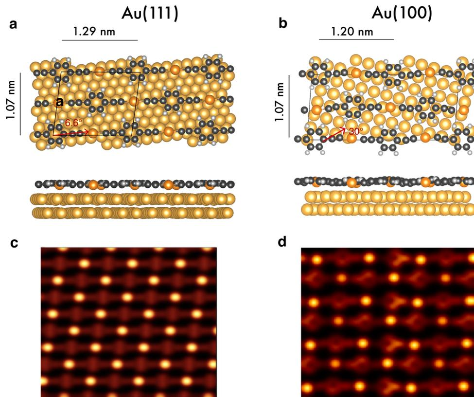
**Fig. 4** Structural model adopted in the calculations for OMW domains on Au(111) (a) and Au(100) (b) and associated STM simulation: OMW on Au(111) (c), and OMW on Au(100) (d), at a bias of +0.5 eV. Red arrows in (a) and (b) mark the  $[1\bar{1}2]$  and  $[011]$  directions, respectively, and the angle described by OMW reported accordingly.
