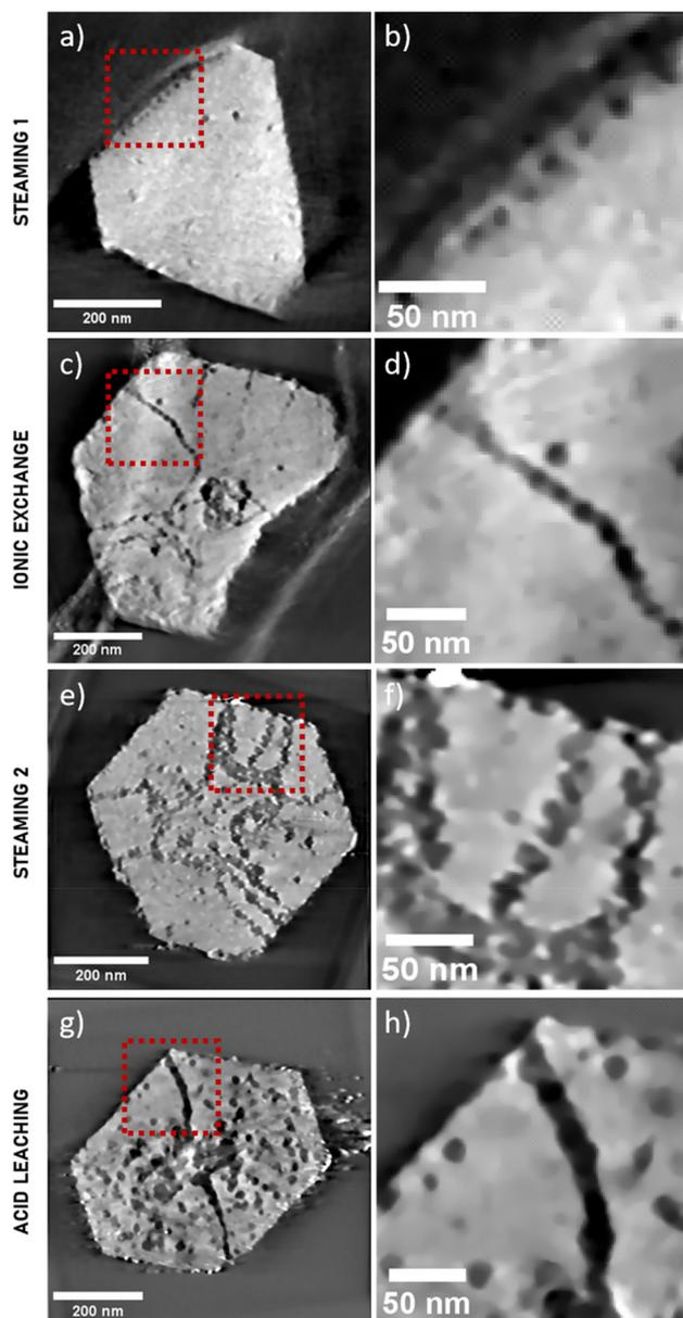
**Fig. 6** Reconstructed slices monitoring the evolution and propagation of the mesoporous morphology within the zeolites at the four steps of the dealuminating treatment: after steaming 1 (a and b), ionic exchange (c and d), steaming 2 (e and f) and acid leaching (g and h).
