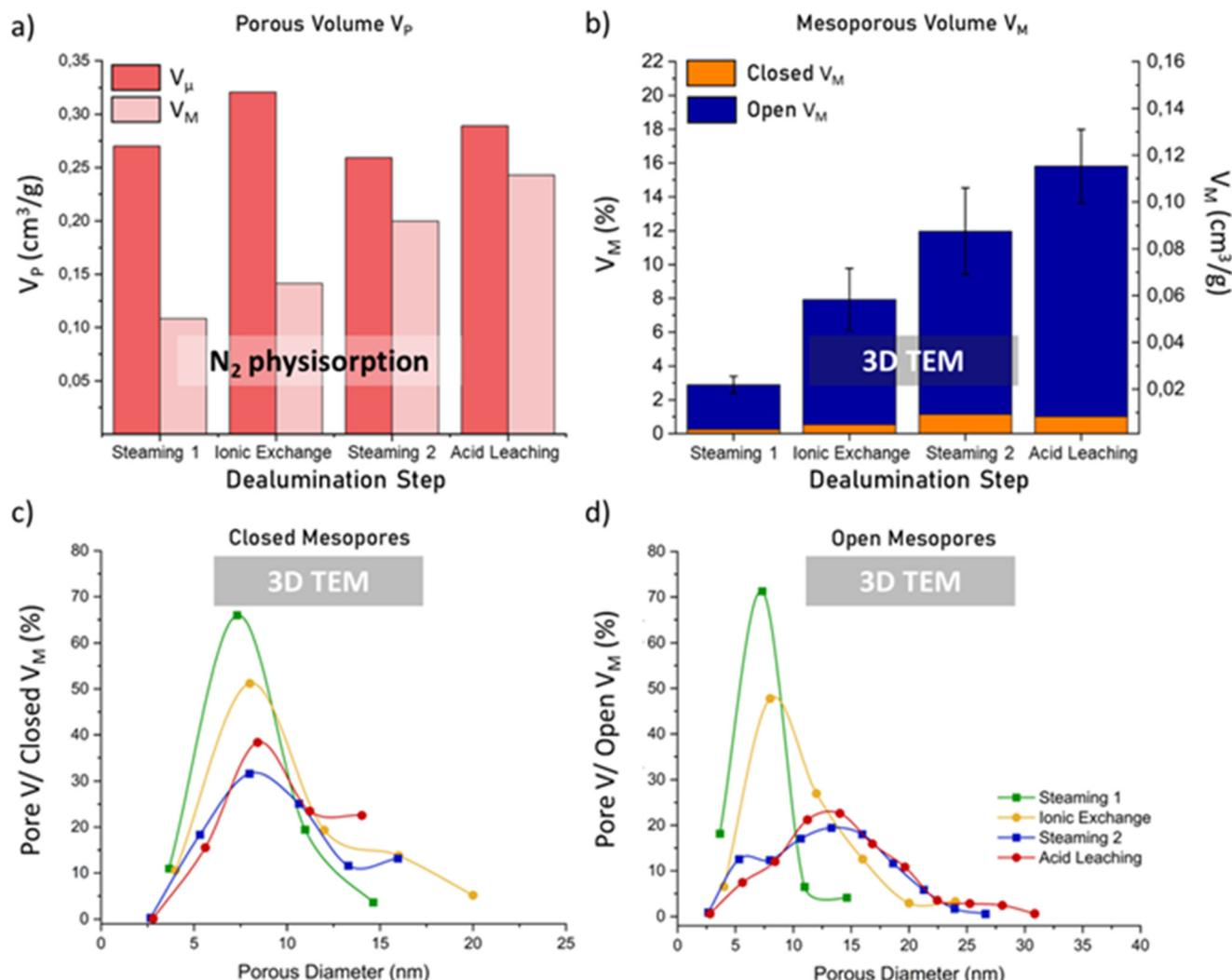
**Fig. 4** Microporous ( $V_\mu$ ) and mesoporous ( $V_M$ ) volumes obtained by N<sub>2</sub> physisorption (a). The sum of  $V_\mu$  and  $V_M$  results in the total porous volume that is accessible during the adsorption and desorption. Mesoporous volume obtained by 3D TEM on individual grains as the sum of the closed (orange) and open (blue) mesoporous volume (b). The discretized PSD derived from 3D TEM for both closed (c) and open (d) porosity along with the dealumination steps.
