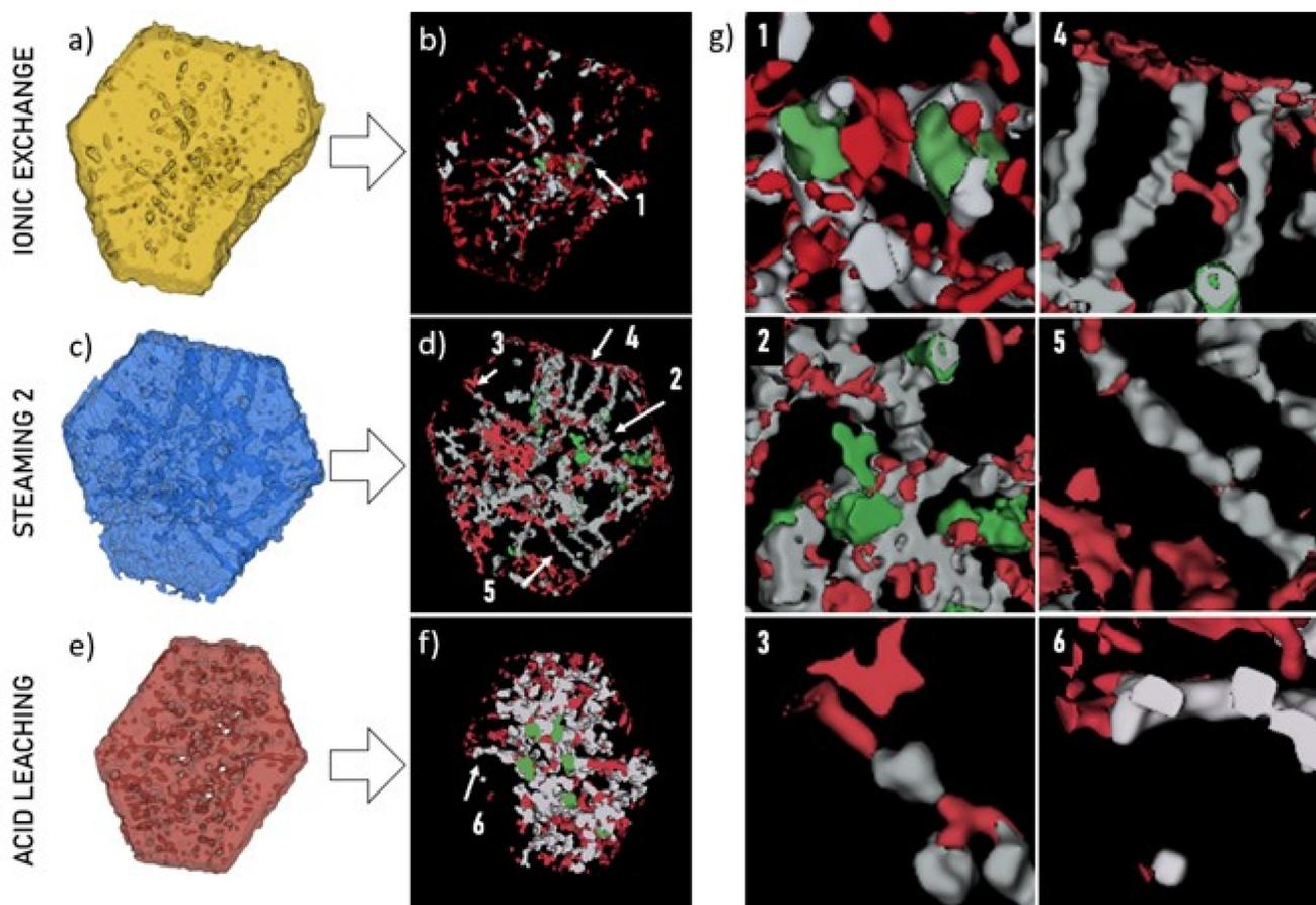
**Fig. 5** 3D volumes of zeolites used for the 3D TEM analysis after the ionic exchange (a), the steaming 2 (c) and the leaching (e) and their corresponding 3D rendering of the mesopores network (b, d and f). The PSD of the open mesopores is divided here into three ranges (g): red ( $d \leq 8$  nm), grey ( $8 < d \leq 20$  nm) and green ( $d > 20$  nm). The zoomed renderings from 1 to 6 of the mesopores correlate the pores morphology with their sizes.
