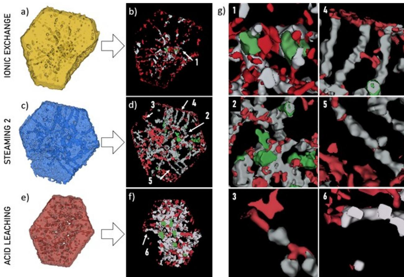
**Fig. 5** 3D volumes of zeolites used for the 3D TEM analysis after the ionic exchange (a), the steaming 2 (c) and the leaching (e) and their corresponding 3D rendering of the mesopores network (b, d and f). The PSD of the open mesopores is divided here into three ranges (g): red ( $d < 8$  nm), grey ( $8 < d \leq 20$  nm) and green ( $d > 20$  nm). The zoomed renderings from 1 to 6 of the mesopores correlate the pores morphology with their sizes.
