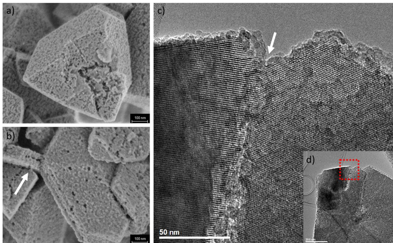
**Fig. 3** SEM images of steaming 1 (a) and acid leached zeolites (b). The surface roughness and the mesoporosity between twinned crystals is already present at the early step of the dealumination. HRTEM micrograph illustrating the presence of a stacking fault in a steaming 2 zeolite (c) and the full field area (d). At more advanced stages in the treatment, such as after a second hydrothermal treatment or a leaching, the mesopores further concentrate on stacking faults (white arrows).
