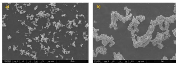
Fig. 7 SEM images of CaO: (a) magnification of 1000 $\times$  at 15.0 kV; (b) magnification of 5000 $\times$  at 5.00 kV.
