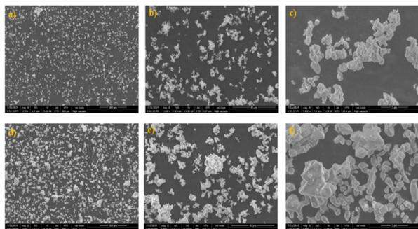
Fig. 10 SEM images (magnification, electron penetration) of KNO<sub>3</sub>/CaO calcined at 700 °C; (a) 250×, 15.00 kV; (b) 1000×, 15.00 kV; (c) 5000×, 5 kV and KNO<sub>3</sub>/CaO calcined at 900 °C; (d) 250×, 15.00 kV; (e) 1000×, 15.00 kV; (f) 5000×, 5.00 kV.
