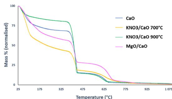
Fig. 11 Thermograms of the heterogenous metal oxide catalyst.
