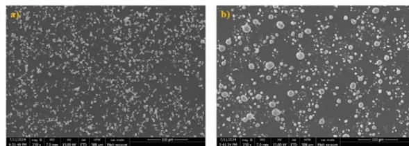
Fig. 6 SEM images (magnification of 250 $\times$  at 15.00 kV) of CaO (a) and MgO (b).
