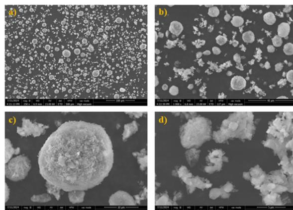
Fig. 8 SEM images of MgO/CaO at 15.00 kV: (a) magnification of 250 $\times$ ; (b) magnification of 1000 $\times$ ; (c) zoomed-in on MgO particles with a magnification of 3000 $\times$ ; (d) zoomed-in on cubic structures with a magnification of 5000 $\times$ .
