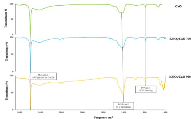
Fig. 5 FT-IR characterisation of the calcined heterogeneous catalysts – CaO, KNO<sub>3</sub>/CaO 700, and KNO<sub>3</sub>/CaO 900.
