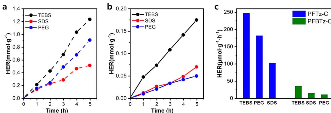
Fig. 2 (a) and (b) Time-dependent photocatalytic hydrogen evolution activities of **PFOTzT** and **PFOTz** nanoparticles obtained using TEBS, PEG, and SDS surfactants. (c) A comparison of the photocatalytic HER activity by surfactant type under AM 1.5G illumination with 1.0 M ascorbic acid (pH 4.0).
