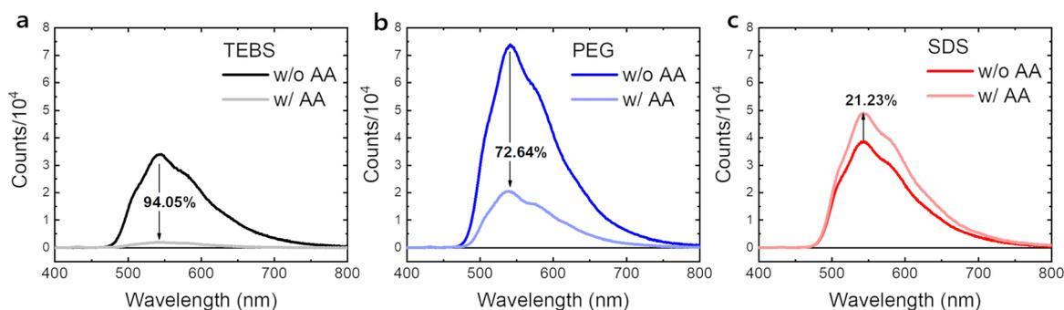
Fig. 4 Steady-state PL spectra of **PFOTzT** nanoparticles stabilized with (a) TEBS, (b) PEG, and (c) SDS, measured before and after ascorbic acid addition.
