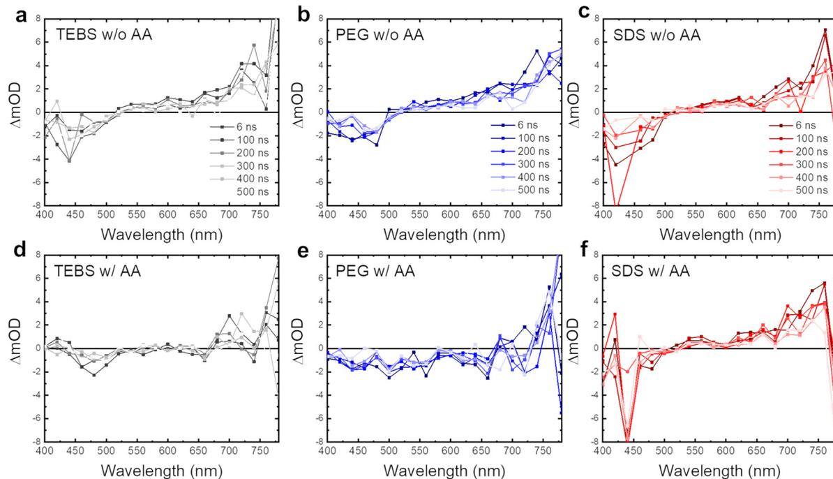
Fig. 5 Transient absorption spectra of **PFOTzT** nanoparticles stabilized with (a) and (d) TEBS, (b) and (e) PEG, and (c) and (f) SDS, measured without AA (a)–(c) and with AA (d)–(f). Spectra were recorded after various delay times (6–500 ns) following 355-nm pulsed excitation.
