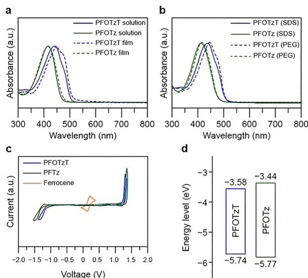
**Fig. 1** UV-vis absorption spectra of the polymers (a) in solution and film states and (b) as nanoparticles prepared *via* mini-emulsion (SDS) and nanoprecipitation (PEG). (c) Cyclic voltammograms of the polymers and (d) HOMO/LUMO energy level diagrams of the polymers in the neutral state from CV and optical band gap measurements.
