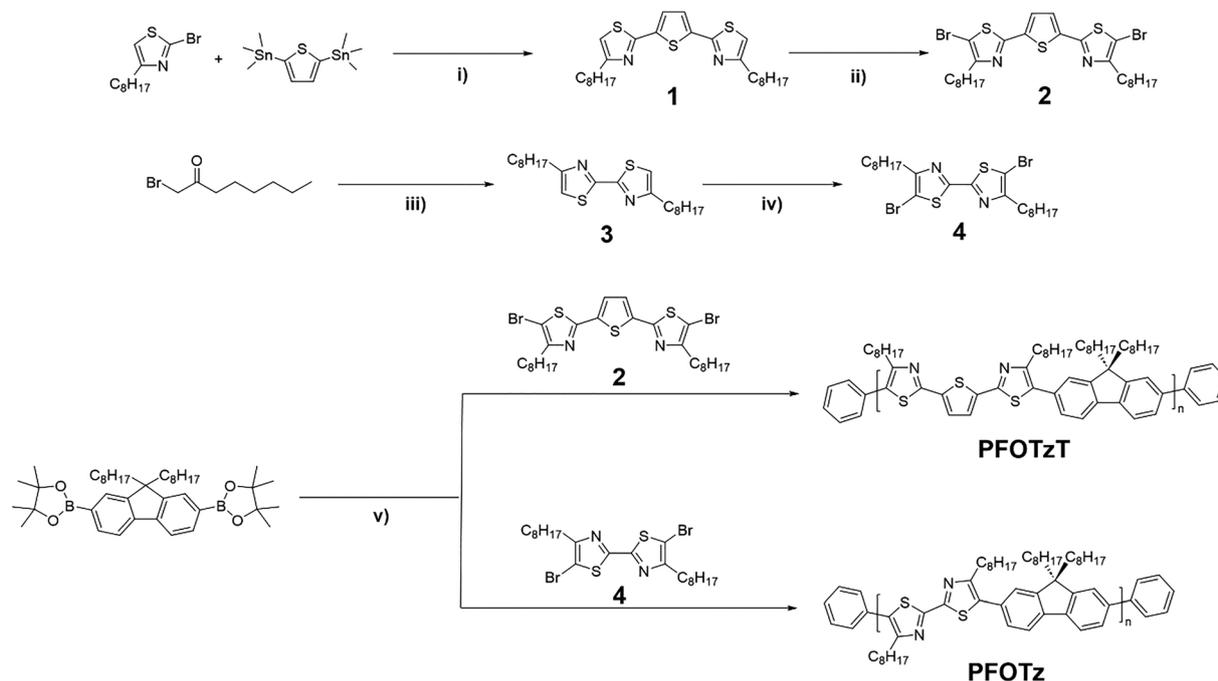
**Scheme 1** Synthetic routes to OTz-based monomers and polymers (**PFOTzT** and **PFOTz**). Reaction conditions: (i) Pd(PPh<sub>3</sub>)<sub>4</sub>, toluene, 110 °C; (ii) NBS, DMF; (iii) dithioamide, dithioamide, ethanol; (iv) NBS, DMF/AcOH; (v) Aliquat 336, Pd(PPh<sub>3</sub>)<sub>4</sub>, 2 M K<sub>3</sub>PO<sub>4</sub>, toluene, 110 °C.
