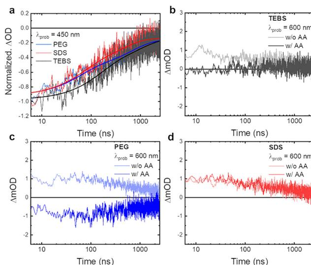
Fig. 6 (a) GSB decay at 450 nm for **PFOTzT** nanoparticles, revealing the exciton lifetime dynamics in the absence of AA. (b)–(d) PIA decay at 600 nm for **PFOTzT** nanoparticles stabilized with TEBS, PEG, and SDS, respectively, measured with and without AA.
