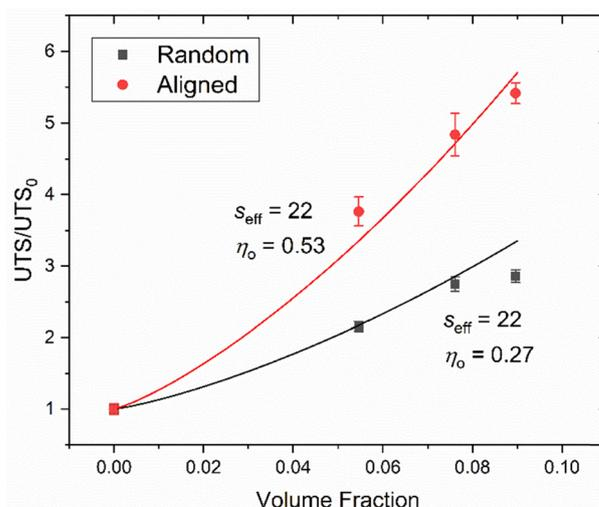
**Fig. 4** UTS of the nanocomposites as a function of MWCNT volume fraction for randomly-oriented or aligned SD-1300 CNTs compared with the UTS of the matrix. The data were fitted to eqn (3) using an  $s_{\text{eff}}$  value of 22.
