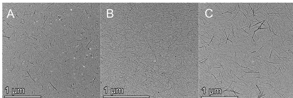
Fig. 1 TEM images of defibrillated samples (A) DEEA-MCC<sup>UT</sup>, (B) DEEA-SBKP<sup>UT</sup>, (C) DEEA-chitin<sup>UT</sup>.
