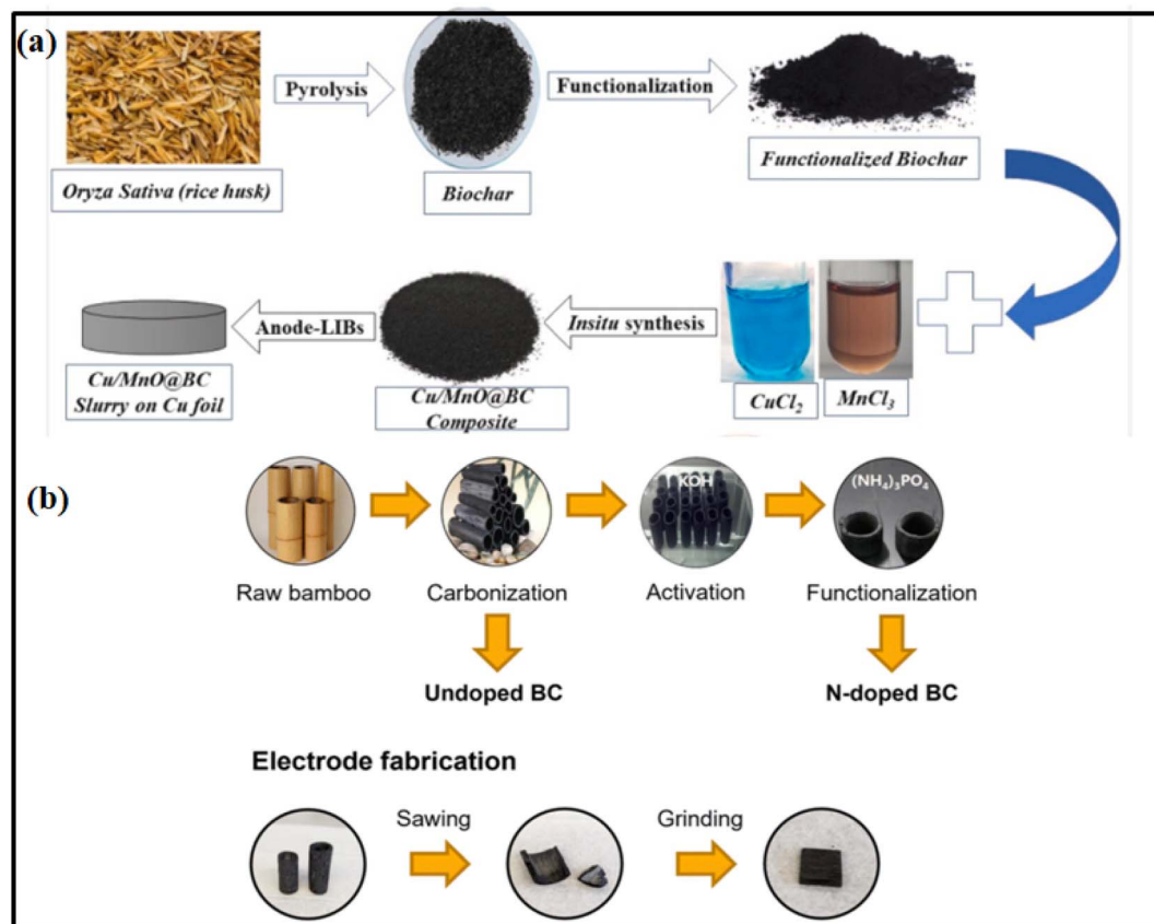
Fig. 4 Schematic of synthesis of (a) rice husk biochar Cu/MnO based nanocomposite 58 adapted from ref. 58 via Creative Commons CC BY-NC-ND 4.0 licence, [Elsevier], copyright 2024 and (b) raw bamboo N-doped biochar for electrode preparation 59 adapted from ref. 58 via Creative Commons CC BY 3.0 licence, [Royal Society of Chemistry], copyright 2024.
