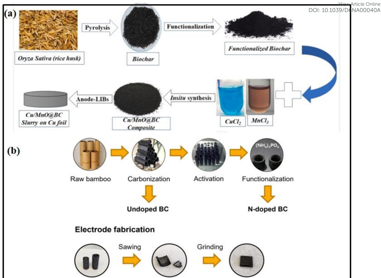
Fig. 4. Schematic of synthesis of (a) rice husk biochar Cu/MnO based nanocomposite 58 adapted from ref 58 via Creative Commons CC BY-NC-ND 4.0 licence, [Elsevier], copyright 2024 and (b) raw bamboo N-doped biochar for electrode preparation 59 adapted from ref 58 via Creative Commons CC BY 3.0 licence, [Royal Society of Chemistry], copyright 2024.
