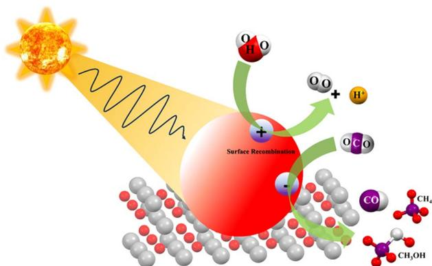
Fig. 6 Photocatalytic CO<sub>2</sub> conversion mechanism in MQD-based composite materials.
