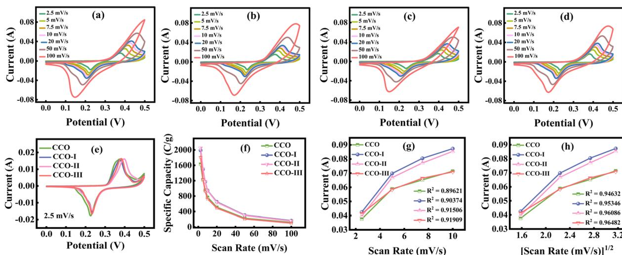
Fig. 3 CV profiles at different scan rates for (a) pristine CCO, (b) CCO-I, (c) CCO-II, and (d) CCO-III, (e) comparison of CV profiles of all samples at 2.5 mV s<sup>-1</sup>, (f) specific capacity of all samples at different scan rates, (g) current vs. scan rate plot for capacitive contribution, and (h) current vs. (scan rate)<sup>1/2</sup> plot for diffusive contribution.
