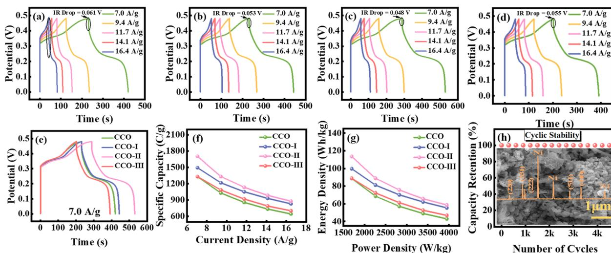
Fig. 6 (a–d) GCD curves of CCO, CCO-I, CCO-II, and CCO-III, respectively, at different current densities, (e) comparison of GCD curves at  $7.0 \text{ A g}^{-1}$ , (f) specific capacity of all samples at different current densities, (g) Ragone plot, and (h) cyclic stability, post-cycling XRD, and SEM image of CCO-II electrode.
