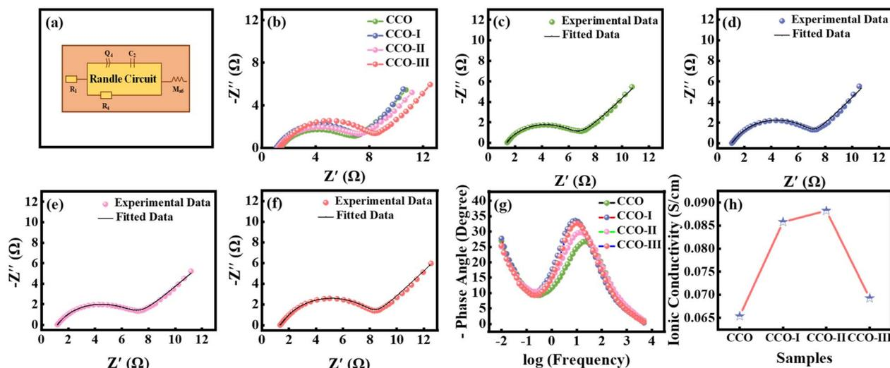
Fig. 8 (a) Resultant Randle circuit, (b) combined Nyquist plot of all samples, (c–f) Nyquist plots of CCO, CCO-I, CCO-II, and CCO-III, respectively, (g) Bode phase plot, and (h) samples vs. ionic conductivity plot.
