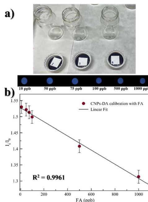
Fig. 6 (a) Real image of the experimental setup. (b) Linear range for gaseous FA sensing between 10 ppb and 1 ppm, with  $R^2 = 0.9961$ ; real images of the spots under a UV LED are reported on the top of the plot.
