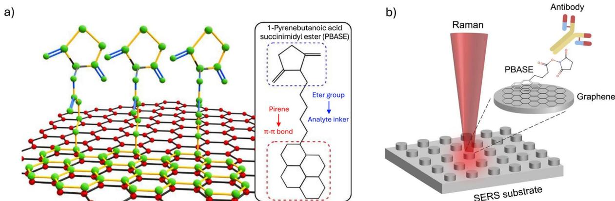
Fig. 1 (a) Molecular representation of PBASE molecules interacting with the graphene surface through  $\pi$ - $\pi$  stacking. The inset shows the molecular structure of PBASE, highlighting the pyrene group responsible for graphene attachment and the succinimide ester group for covalent bonding to the antibody. (b) Schematic illustration of the hybrid SERS platform based on an array of silicon nanopillars on silica coated with a graphene monolayer functionalized with PBASE.
