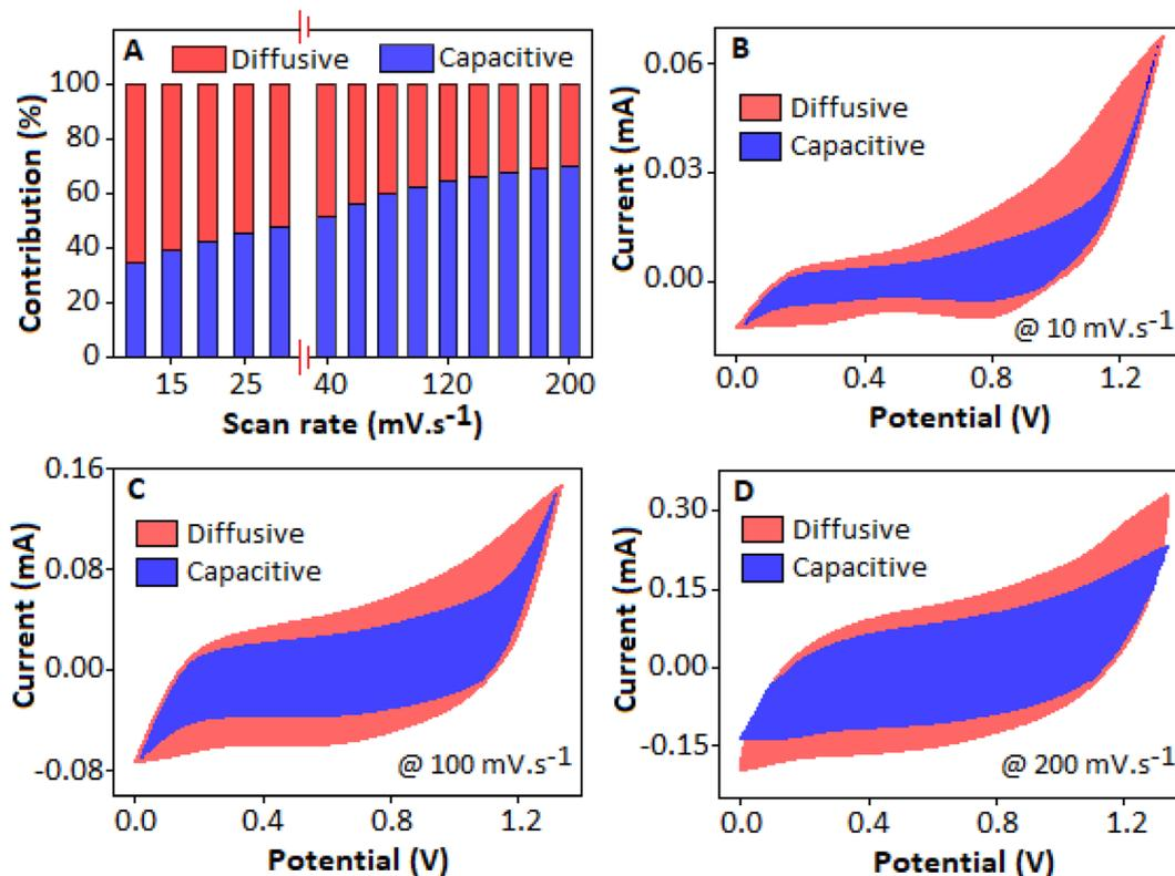
Fig. 10 (A) Bar diagram for the capacitive and diffusive contributions of the device at different scan rates from  $10 \text{ mV s}^{-1}$  to  $200 \text{ mV s}^{-1}$ . (B–D) Capacitive and diffusion contributions based on the experimental CV curves at 10, 100 and  $200 \text{ mV s}^{-1}$  respectively.
