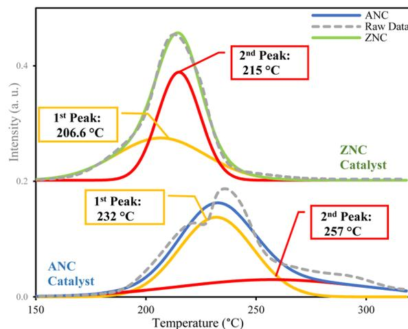
**Fig. 6** H<sub>2</sub>-TPR profiles of both catalysts.
