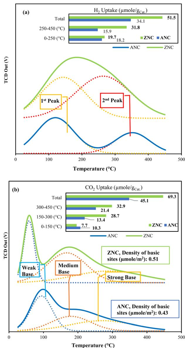
Fig. 7 (a) H<sub>2</sub>-TPD and (b) CO<sub>2</sub>-TPD profiles: comparative analysis of basicity and hydrogen uptake in ZNC and ANC catalysts.
