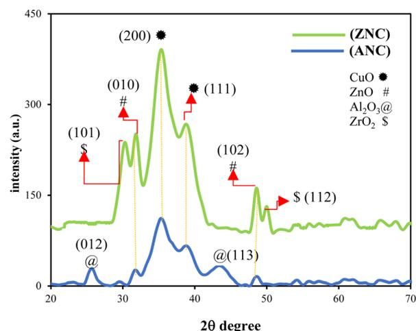
Fig. 3 X-ray diffraction patterns of ANC and ZNC catalysts.
