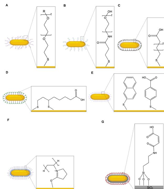
Fig. 4 Self-assembly with various surface ligands on AuNRs to facilitate the MOF shell growth. The ligands or MN used to be functionalized with AuNRs to date are: (A) HS-PEG; (B) HS-(CH<sub>2</sub>)<sub>2</sub> CO-NH-PEG-OH; (C) MUA; (D) LA; (E) NPT (left) and MBA (right); (F) PVP; and (G) MSN-COOH.
