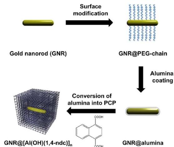
Fig. 9 Schematic of the synthesis of AuNR@[Al(OH)(1,4-ndc)]<sub>n</sub> core-shell composites. Reproduced from ref. 38. Copyright 2013 ACS Publications.
