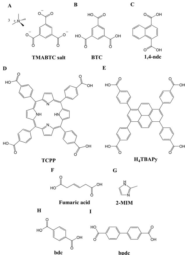
Fig. 6 Chemical structures of the organic linkers: (A) TMABTC salt; (B) BTC; (C) 1,4-ndc; (D) TCPPP; (E) H<sub>4</sub>TBAPy; (F) fumaric acid; (G) 2-MIM; (H) bdc; and (I) bpdc.
