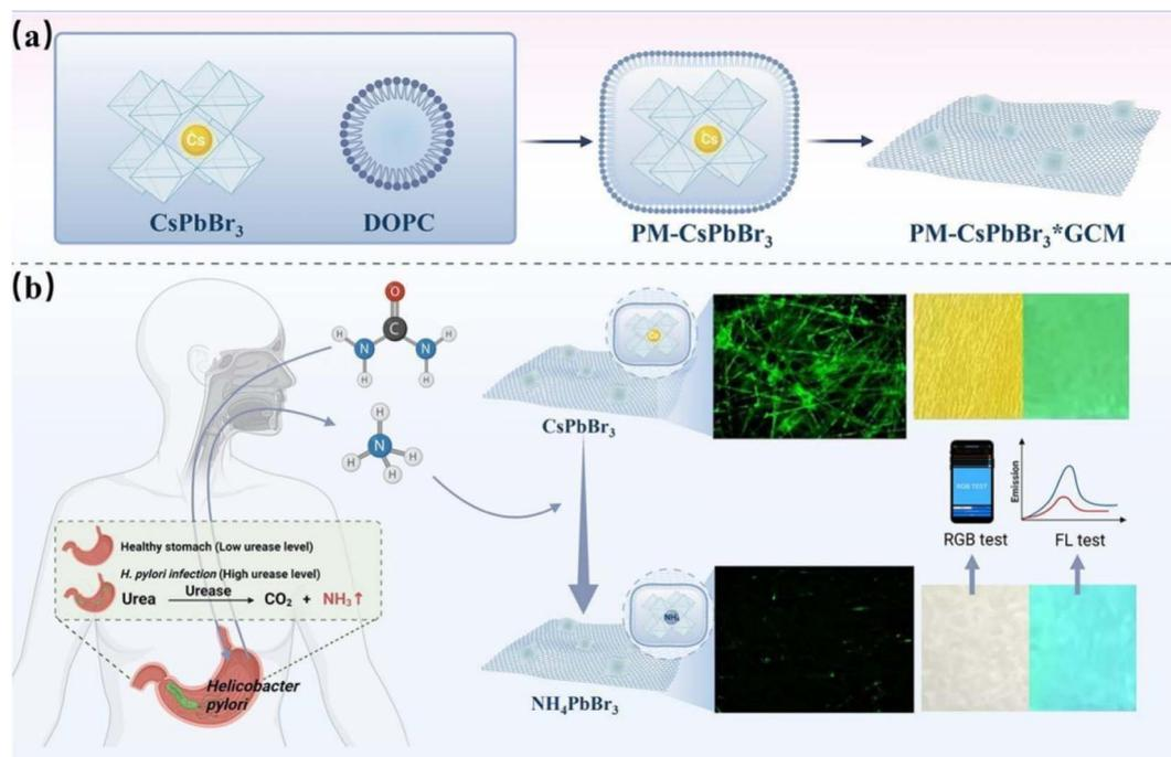
Fig. 4 (a) PM-CsPbBr<sub>3</sub>\*GCM sensor fabrication: CsPbBr<sub>3</sub> QDs in DOPC, electrospun onto glass cellulose membrane. (b) *H. pylori* detection: sensor detects breath ammonia with fluorescence quenching and color shift (yellow to green). Reproduced with permission from Yang *et al.*, *Microchem. J.*, 2025, **212**, 113–263. © Elsevier 2025.
