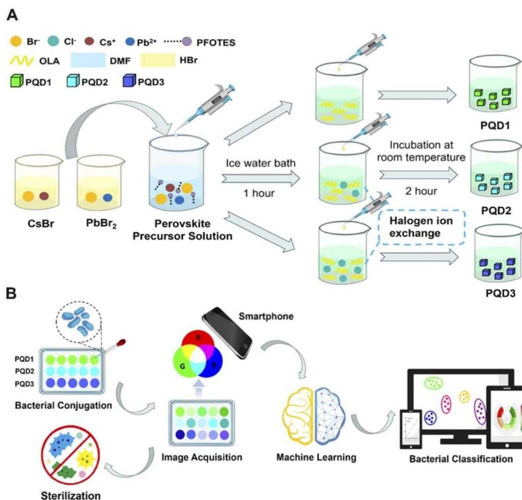
Fig. 6 (A) CsPbBr<sub>3</sub> QD synthesis: CsBr/PbBr<sub>2</sub>, ice bath (1 h) for PQD1, room temp (2 h) for PQD2, halogen exchange for PQD3. (B) QD use: pathogen detection *via* conjugation, smartphone imaging, SVM (100% accuracy,  $1.0 \times 10^3$ – $10^7$  CFU mL<sup>-1</sup>), and >99% inactivation in 30 min. Reproduced with permission from Zhang *et al.*, *J. Hazard Mater.*, 2025, **483**, 136 655. © Elsevier 2025.
