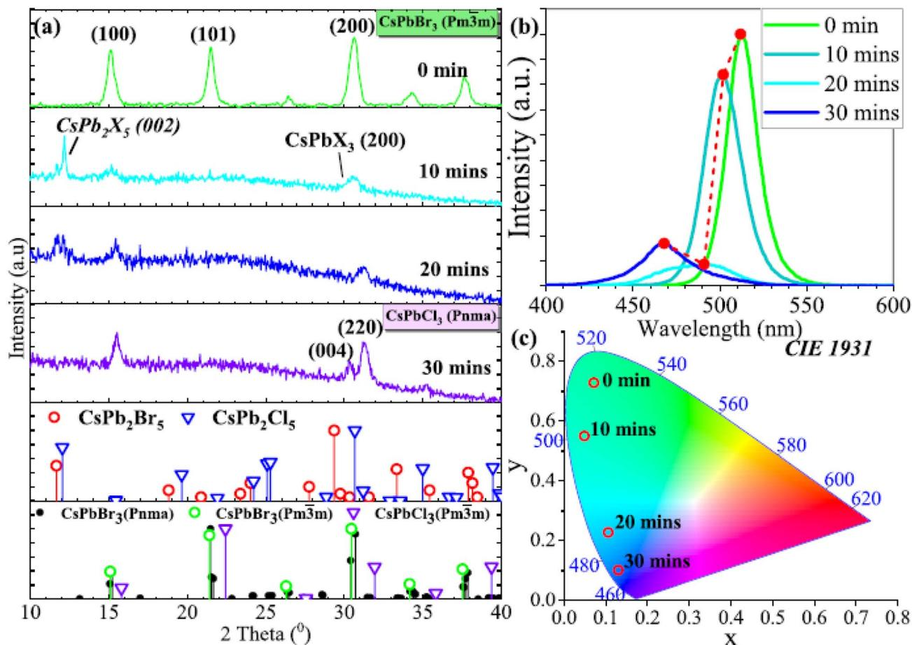
Fig. 10 (a) XRD analysis of CsPbBr<sub>3</sub> PQDs thin film exposed to 5% NaOCl under UV light at 0, 10, 20, and 30 minutes. (b) Fluorescence spectra of CsPbBr<sub>3</sub> PQDs thin film at 0, 10, 20, and 30 minutes. (c) CIE 1931 color space coordinates of CsPbBr<sub>3</sub> PQDs thin film at 0, 10, 20, and 30 minutes. Reprinted with permission from ref. 91, Copyright 2025 American Chemical Society.
