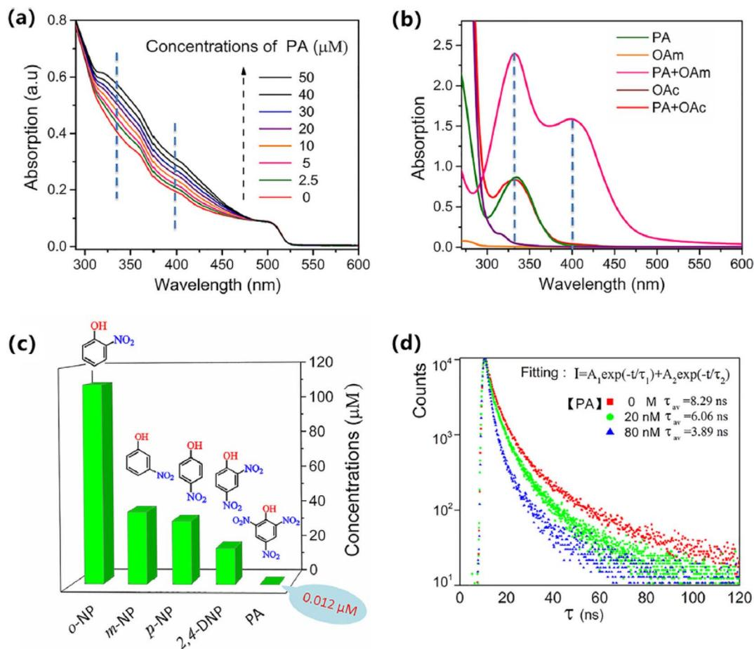
Fig. 9 (a) UV-vis absorption spectra of CsPbBr<sub>3</sub> PQDs with varying PA concentrations (0–50 μM). (b) UV-vis absorption spectra of PA, OAm, OAc, PA + OAm, and PA + OAc mixtures. (c) Concentrations of phenolic hydroxyl compounds (PA, 2,4-DNP, *p*-NP, *m*-NP, *o*-NP, Ph) required for half fluorescence quenching. (d) Fluorescence decay curves of CsPbBr<sub>3</sub> PQDs with PA concentrations (0, 20, 80 nM). Reprinted from ref. 87, Copyright 2020, with permission from Elsevier.
