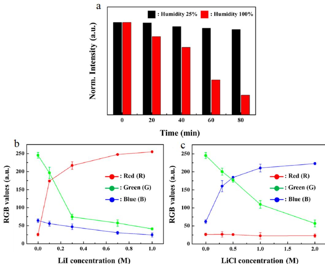
Fig. 8 (a) Normalized intensity of CsPbBr<sub>3</sub> PQDs/cellulose composites under UV illumination ( $\lambda_{\text{ex}} = 365$  nm) at 25% (black) and 100% (red) humidity over time. (b) RGB values (Red, Green, Blue) as a function of iodide concentration. (c) RGB values as a function of chloride concentration. Reprinted with permission from ref. 85, Copyright 2019 American Chemical Society.
