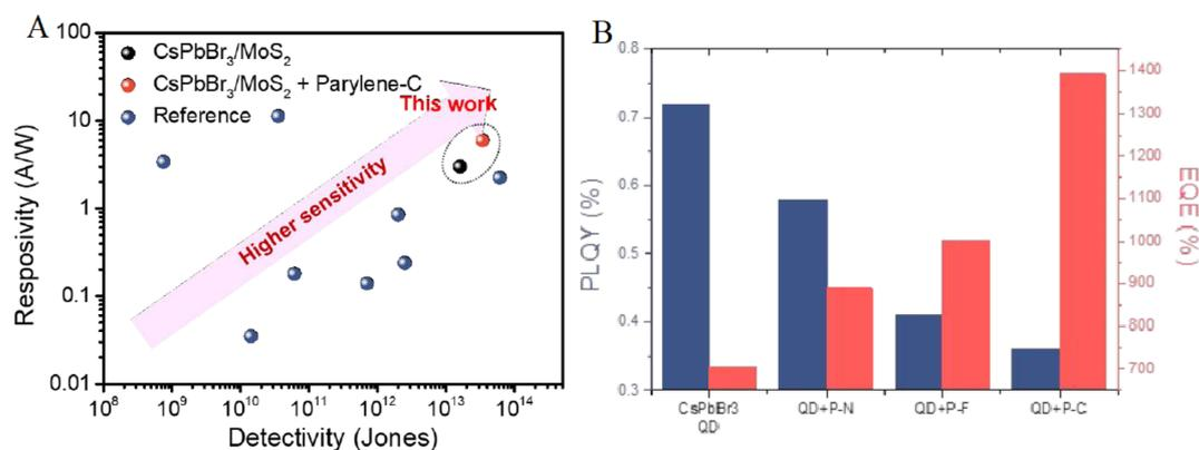
Fig. 5 (A) Responsivity and detectivity comparison of CsPbBr<sub>3</sub>/MoS<sub>2</sub> photosensors with parylene-C coating versus reference. (B) PLQY and EQE of CsPbBr<sub>3</sub> photosensors pre- and post-passivation. Reprinted with permission from ref. 66, Copyright 2023 American Chemical Society.
