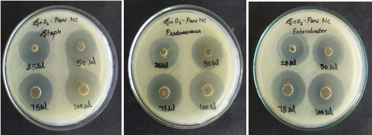
Fig. 20 Zone of inhibition of SnO 2 -PANI Nanocomposite using various bacterial strains and standard antibiotic ciprofloxacin
