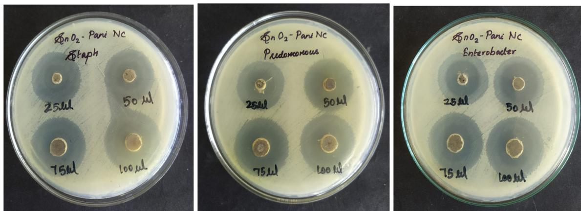
Fig. 20 Zone of inhibition of the SnO<sub>2</sub>-PANI nanocomposite using various bacterial strains.
