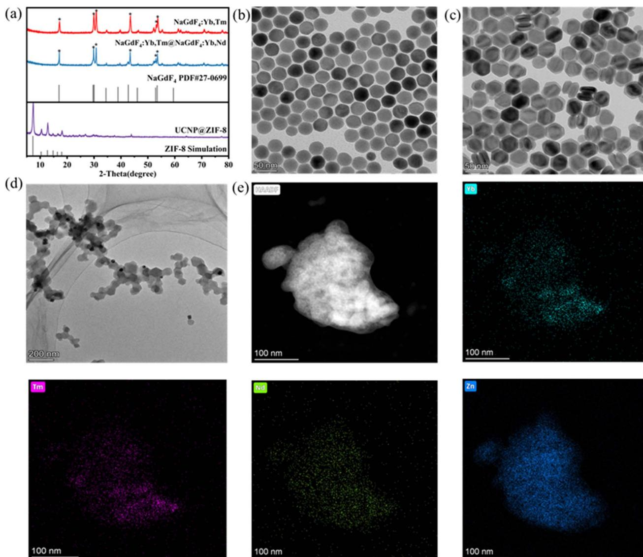
Fig. 1 (a) XRD pattern of the nanomaterials; (b) TEM image of NaGdF<sub>4</sub>:Yb,Tm; (c) TEM image of NaGdF<sub>4</sub>:Yb,Tm@NaGdF<sub>4</sub>:Yb,Nd; (d) TEM image of UCNP@ZIF-8; (e) elemental distribution characterization.
