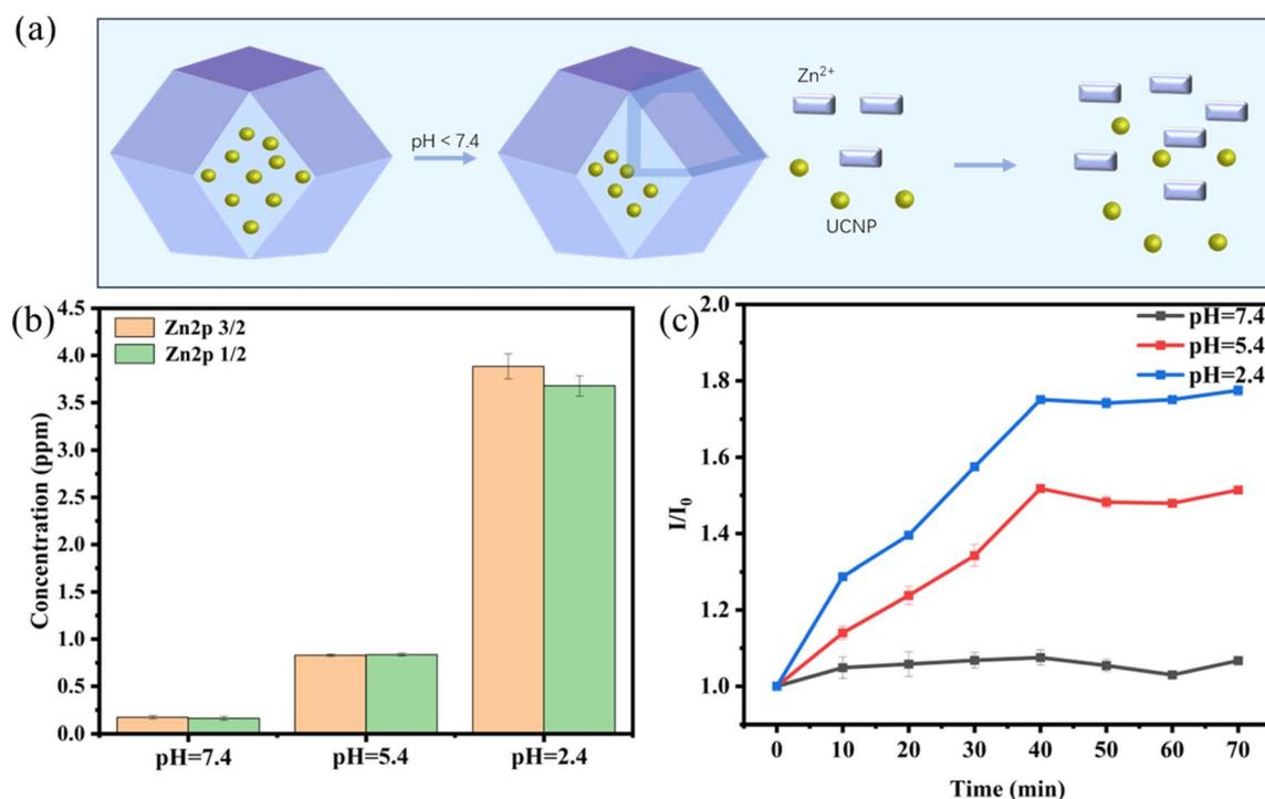
Fig. 5 (a) Schematic diagram of UCNP@ZIF-8 cracking under acidic conditions; (b)  $Zn^{2+}$  concentration in different pH solutions; (c) recovery of the luminescence intensity of the UCNPs under different pH environments.
