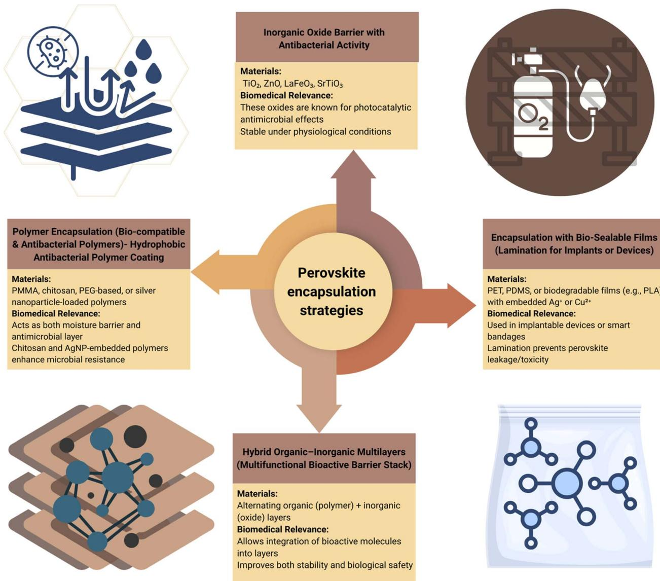
Fig. 12 Figure summarizing various encapsulation strategies employed in perovskite nanocrystals.
