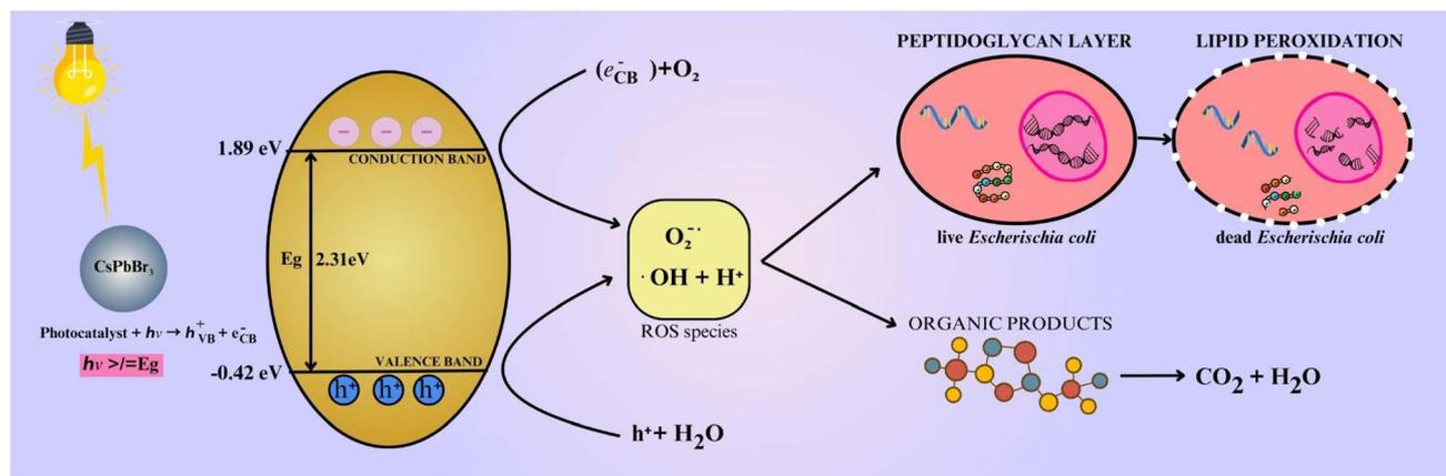
Fig. 3 Schematic representation of ROS-mediated antibacterial action of CsPbBr<sub>3</sub> perovskite under visible light irradiation. Upon photoexcitation ( $E_g = 2.31$  eV), photogenerated electrons and holes facilitate the generation of reactive oxygen species ( $O_2^{\cdot-}$ ,  $\cdot OH$ ), which disrupt the peptidoglycan layer and induce lipid peroxidation, leading to *Escherichia coli* cell death and mineralization of organic products to  $CO_2$  and  $H_2O$ .
