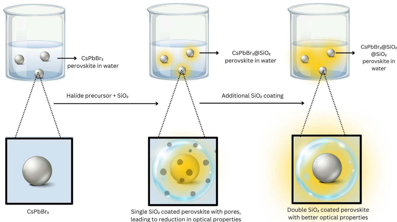
Fig. 13 Schematic diagram showing double SiO<sub>2</sub>-coated perovskites.
