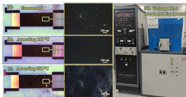
Fig. 5 Actual images of SAW chips and magnetic films (a) unannealed, (b) annealed at 100 °C, (c) annealed at 200 °C, (d) vacuum heat treatment device diagram.
