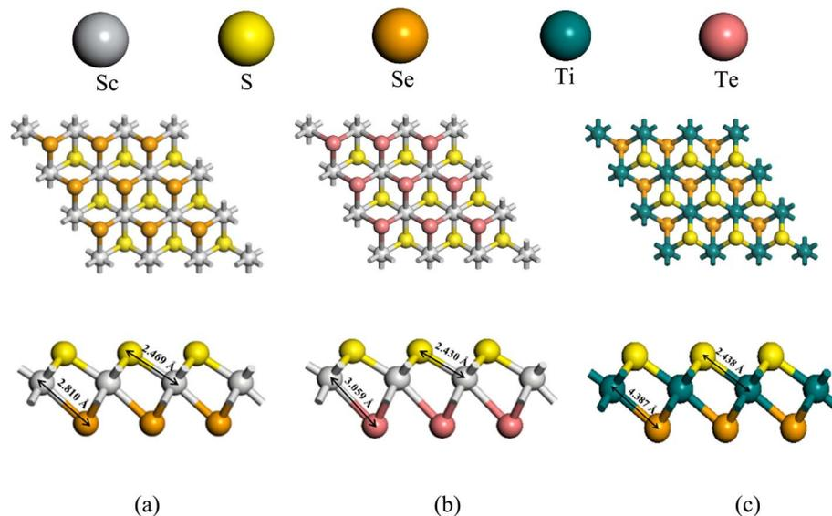
Fig. 1 Top and side views of the optimized structure of (a) ScSeS, (b) ScTeS, and (c) TiSeS.
