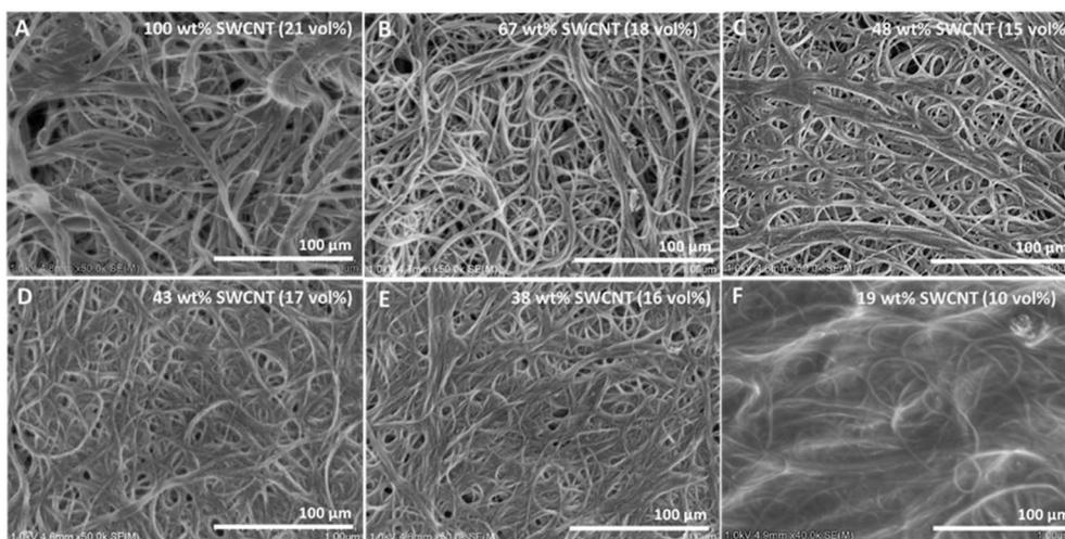
Fig. 3 Representative SEM images of (A) SWCNT-BP and (B–F) SWCNT-TPU nanocomposite sheets of different compositions prepared with the CHCl<sub>3</sub>/methanol mixture (see Table S1 for compositional details).
