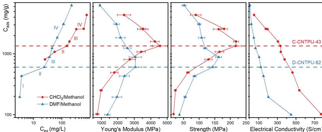
Fig. 6 Correlation between the identified regions of adsorption with mechanical and electrical conductivity trends as a function of the amount of TPU adsorbed by SWCNT ( $\text{mg g}^{-1}$ ). Dashed lines to indicate TPU/SWCNT ratios by the end of region II and solid lines to guide the eyes.
