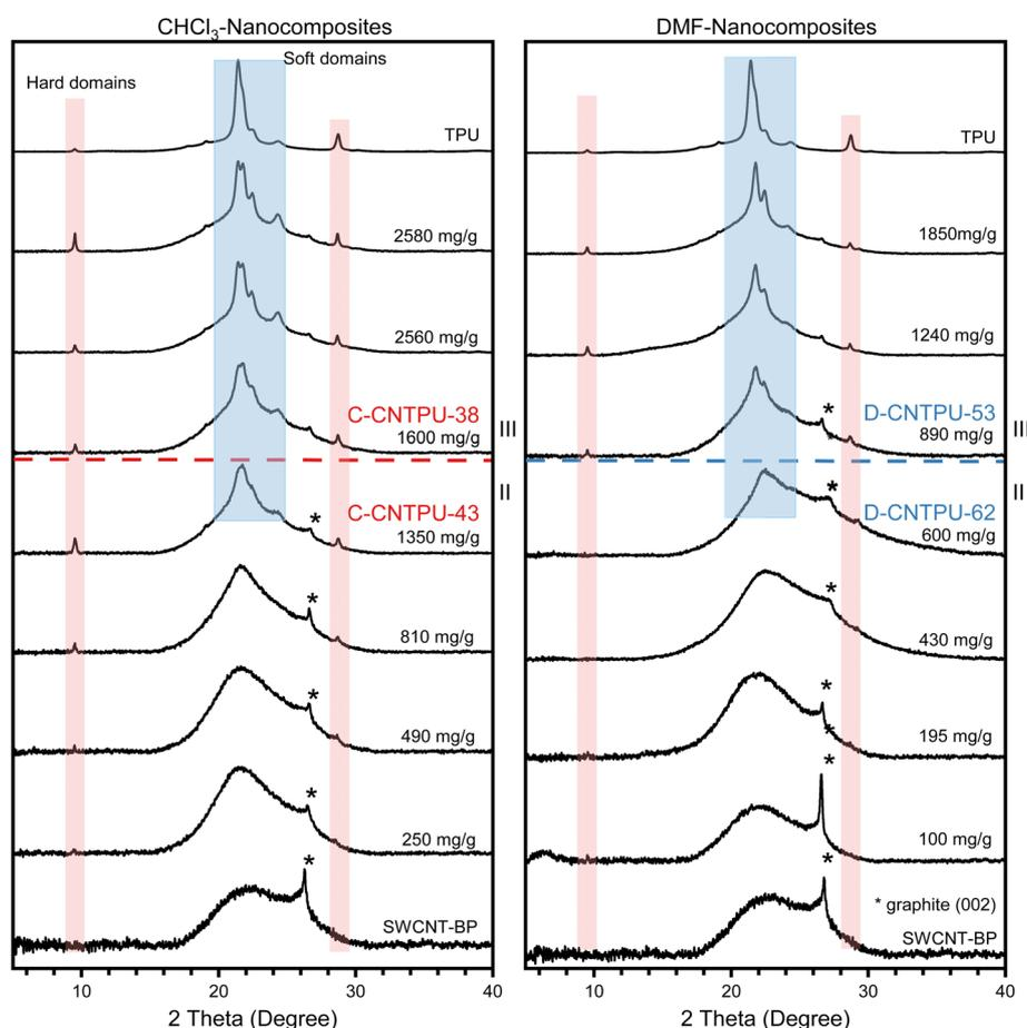
Fig. 8 XRD patterns of TPU, SWCNT-BP, and SWCNT-TPU nanocomposite sheets fabricated using different TPU solvents (DMF and  $\text{CHCl}_3$ ) with methanol as the nonsolvent. Dashed lines to indicate TPU/SWCNT ratios ( $\text{mg g}^{-1}$ ) by the end of region II and transition to region III, corresponding to samples in the optimal mechanical properties range in Fig. 2 and 6. (e.g., C-CNTPU-43 and D-CNTPU-62 in Table S1).
