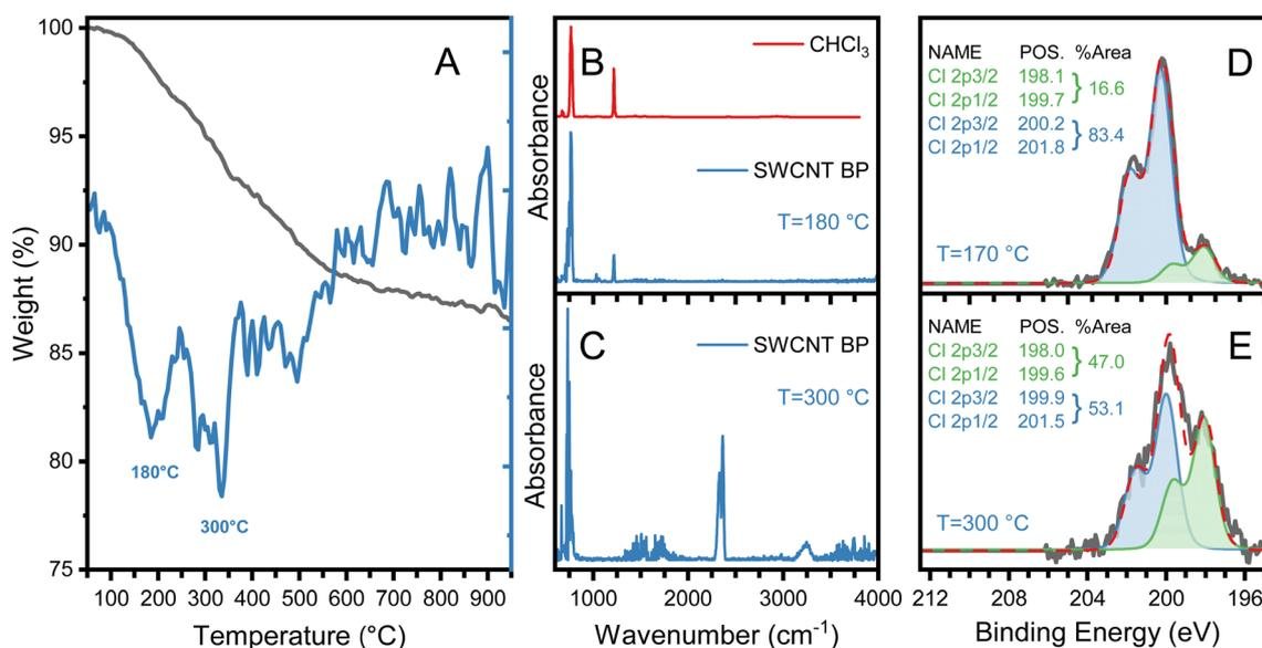
Fig. 4 (A) TG (black) and DTG (blue) under desorption conditions for the SWCNT-BP prepared with  $\text{CHCl}_3$ /methanol. (B) IR absorption spectrum of the species desorbed at 180 °C and the reference gas phase spectrum of  $\text{CHCl}_3$ . (C) IR absorption spectra of the species desorbed at 300 °C. (D) and (E) XPS spectra (Cl 2p lines) for the SWCNT-BP after thermal treatments at 170 °C and 300 °C, respectively.
