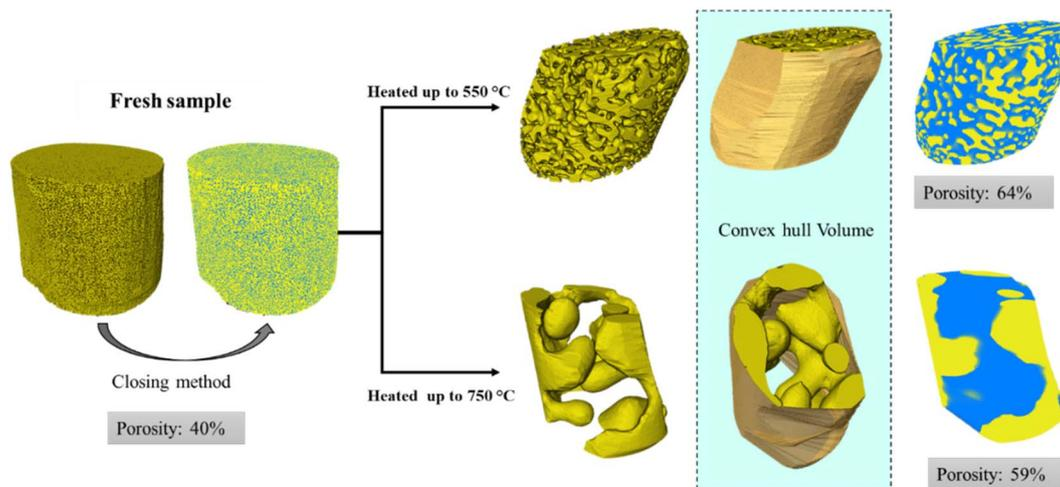
Fig. 1 Summary of tomography data processing, including morphological closing (fresh samples), or convex hull generation and segmentation with labelling of solid and pore phases (thermally treated samples).
