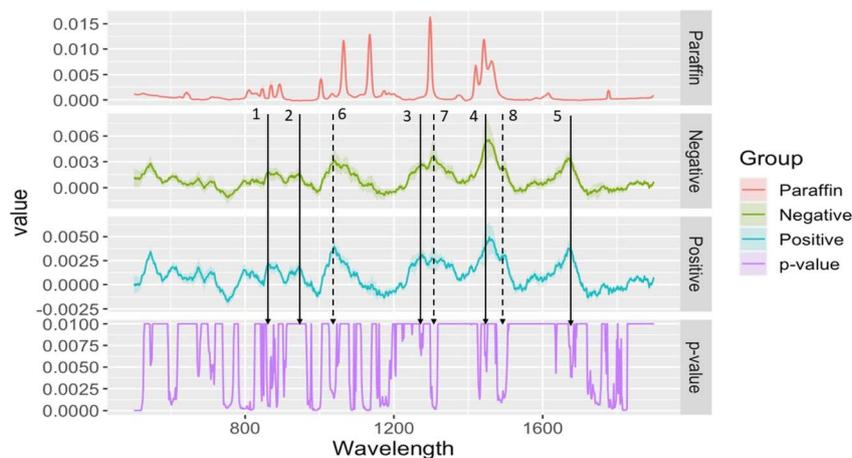
Fig. 3 Au-enhanced average spectra of negative (150 spectra in total) and positive (150 spectra in total) tissue samples acquired using a portable Raman spectrometer with *P*-value of *t*-test. Shaded areas around the average spectra showed the standard deviation of all the spectra in the group. Peaks labeled are listed in Table 1.
