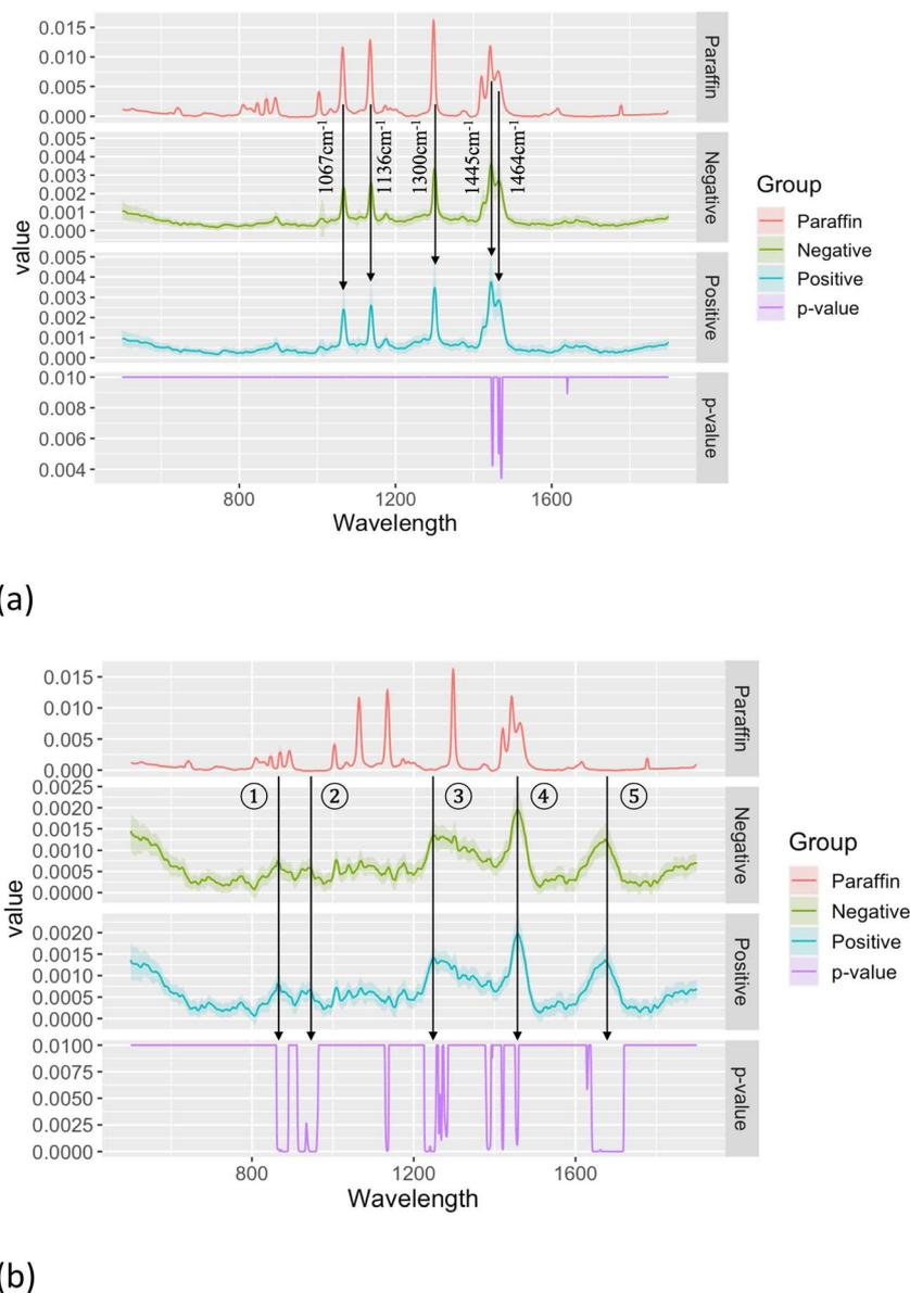
Fig. 2 Average spectra of negative (260 spectra in total) and positive (220 spectra in total) PSS of set A with  $p$ -value of  $t$ -test. (a) Before de-paraffin; (b) after de-paraffin. Shaded areas around the average spectra showed the standard deviation of all the spectra in the group. Peaks labeled in (b) are listed in Table 1.
