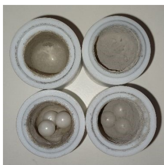
Figure 4 : Rheology after the milling of 1a with 5.0 mL (left) and 6.0 mL (right) of sand. 14 mL PTFE jar was filled with (RS)-2, sand, 2.0 equiv. of Na 2 SO 4 , three ZrO 2 balls of 10 mm of diameter, 1.3 equiv. of DBU and 1.0 equiv. of benzaldehyde.
