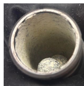
Figure 1: Solid 18-crown-6 adduct of 5a . (for better representation the silanide was made in a 25 mL milling jar with 2 balls instead of a 10 mL milling jar with 1 ball)
