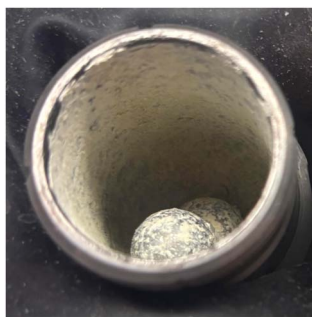
Fig. 1 Solid 18-crown-6 adduct of 5a. (for better representation the silanide was made in a 25 mL milling jar with 2 balls instead of a 10 mL milling jar with 1 ball).
