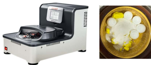
Fig. 2 Planetary ball mill used in this study: Fritsch Pulverisette 7 premium line (left), ZrO 2 bowl before grinding (right).
