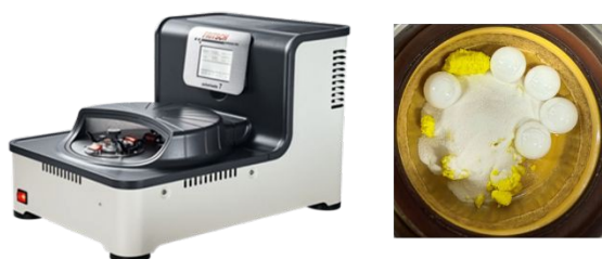
Figure 2. Planetary ball mill used in this study: Fritsch Pulverisette 7 premium line (left), ZrO 2 bowl before grinding (right).
