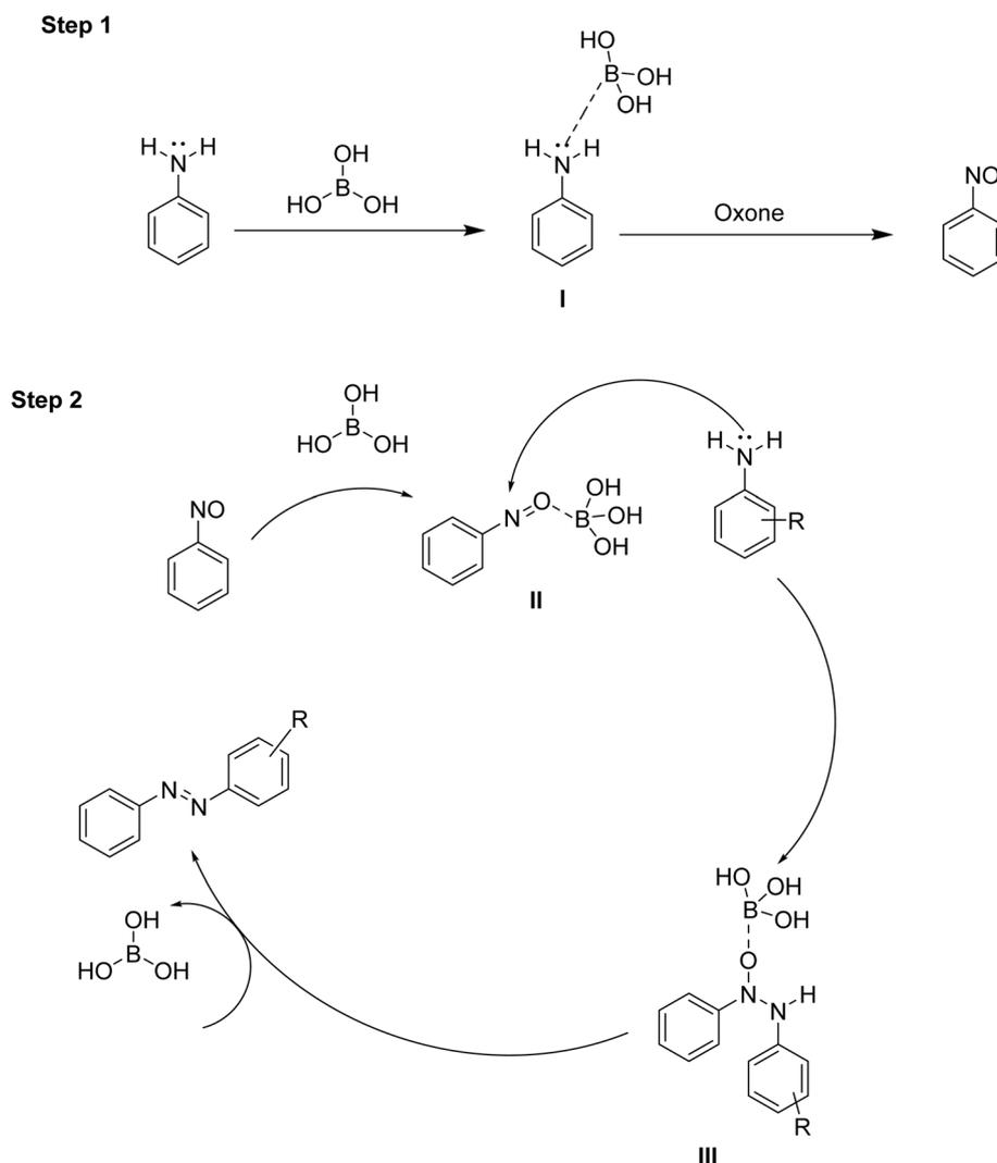
Scheme 3 Probable mechanism for the preparation of azobenzene.
