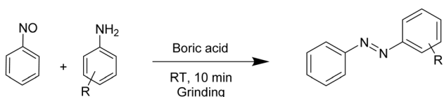
Scheme 2 Synthesis of unsymmetrical azobenzene from amines and nitrosobenzene.
