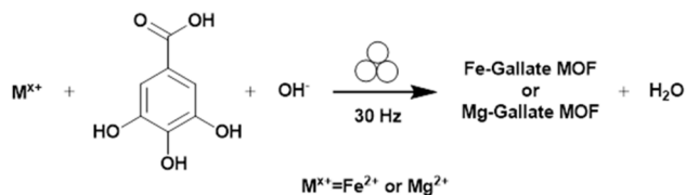
Fig. 1 Mechanochemical synthesis of gallate-based MOFs.
