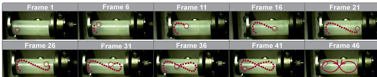
Fig. 3 Series of frames to depict the movement of a 10 mm ball inside a 14 mL PFA vessel. Every fifth frame was used; the position of the ball in the previous frames is indicated by red dots. The ball is outlined in red in the current frame. In the last frame (frame 46), the movement is shown again schematically.
