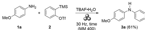
Scheme 2 Test reaction for optimising the mechanochemical conditions.
