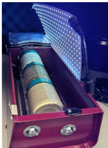
Fig. 1 Photo of scalable mechanochemical synthesis featuring a high-capacity milling chamber with a glass jar affixed to a rock tumbler and incorporated LED lights (365 nm).
